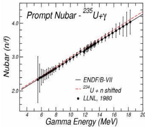
Fig.7. Average number of prompt neutrons emitted per fission (prompt nubar) from  $^{235}\text{U}$  bombarded with photons up to 20 MeV.
