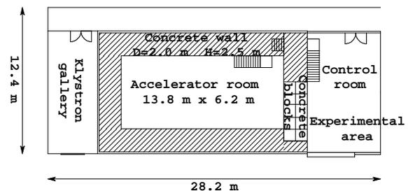
Fig. 1 A schematic drawing of the KU-FEL facility.
