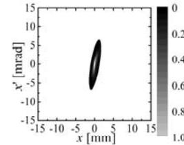
Fig. 10 Phase space distribution with the IEA method at the entrance of Q1.
