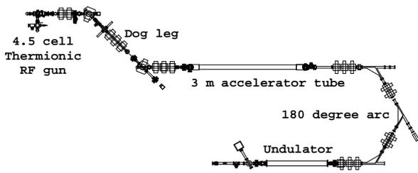
Fig. 2 Arrangement of the KU-FEL.
