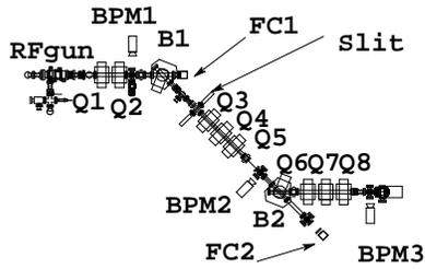
Fig.7 Experimental setup for the analysis of the phase space distribution of the electron beam.
