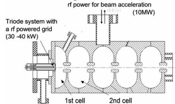
Fig. 16. Concept of the triode thermionic rf gun which have the additional rf cavity at the thermionic cathode.
