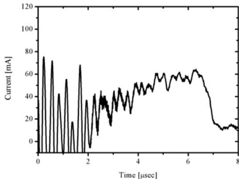
Fig. 5 Beam current measured with CT2
