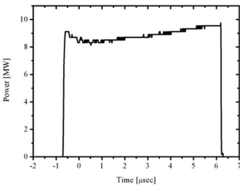
Fig. 4 Waveform of the amplitude modulated rf power fed to the rf gun
