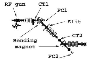
Fig. 3 Experimental setup for the measurement of the beam properties of the energy compensated electron beam.
