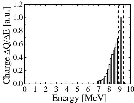
Fig. 8 Energy distribution of the electron beam from the rf gun measured using B1, slit and FC2.
