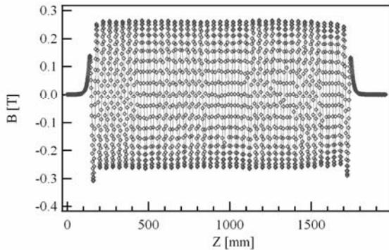
Fig. 11 Measured magnetic field of the undulator along the electron beam axis.
