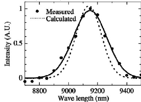
Fig. 15. Measured and calculated spectra of the spontaneous radiation.
