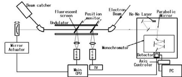
Fig. 14 Experimental setup for the measurement of the spontaneous radiation
