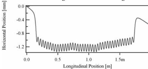
Fig. 12 Horizontal trajectories calculated from the measurement with deflection by the steering magnet located at the entrance of the undulator.
