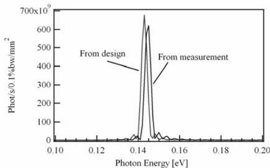
Fig. 13 Calculated spectra of the spontaneous radiation for the designed and the measured magnetic field.
