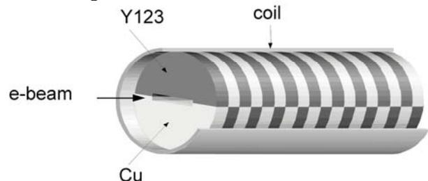
Fig. 17. Conceptual drawing of the high  $T_c$  SC undulator. High  $T_c$  superconducting materials and nonmagnets are stacked in the solenoid.
