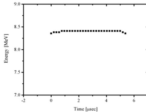
Fig. 6 Measured time evolution of the peak beam energy for the amplitude modulated rf input
