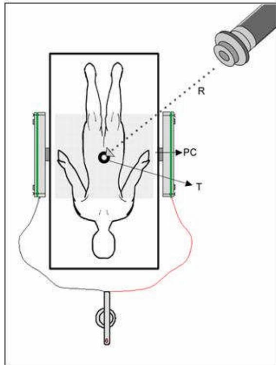
Figure 4 – A proposed new radiotherapy facility, where an external electric field is provided by a capacitor sandwiching the patient.
