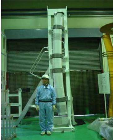
Fig. 4. Ceramic duct for bending magnet is shown.
