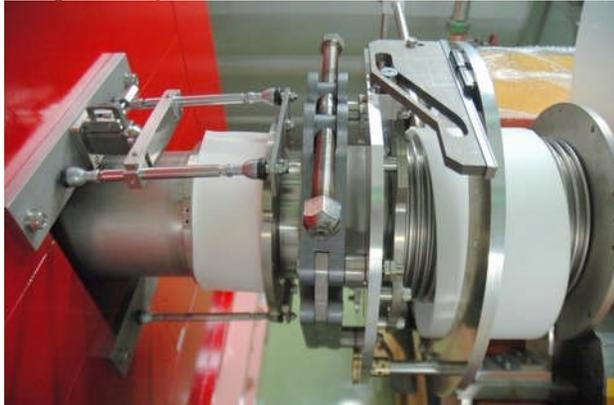
Fig. 11. Semi-remote flange installed at exit of the beam transport (BT) line collimator.
