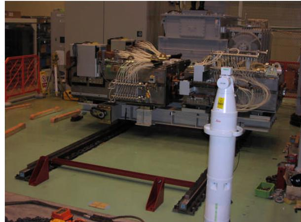
Fig. 9. Septum magnet installed on the linear motion guide.
