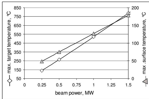
Fig. 14. Temperatures within a rotating segmented target as a function of the beam power at 6 rpm.
