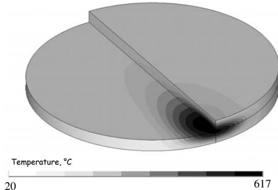
Fig. 9. Stationary temperature distribution inside a monolithic solid tungsten target
