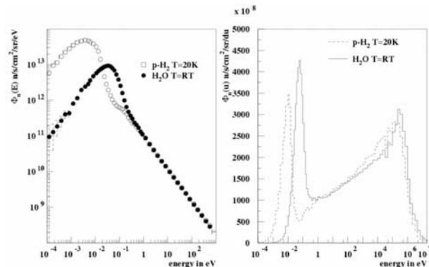
Fig. 5. Energy spectra (left histogram) and lethargy spectra (right histogram) of a water moderator at room temperature and a cold para hydrogen moderator operated at  $T = 20 \text{ K}$ .
