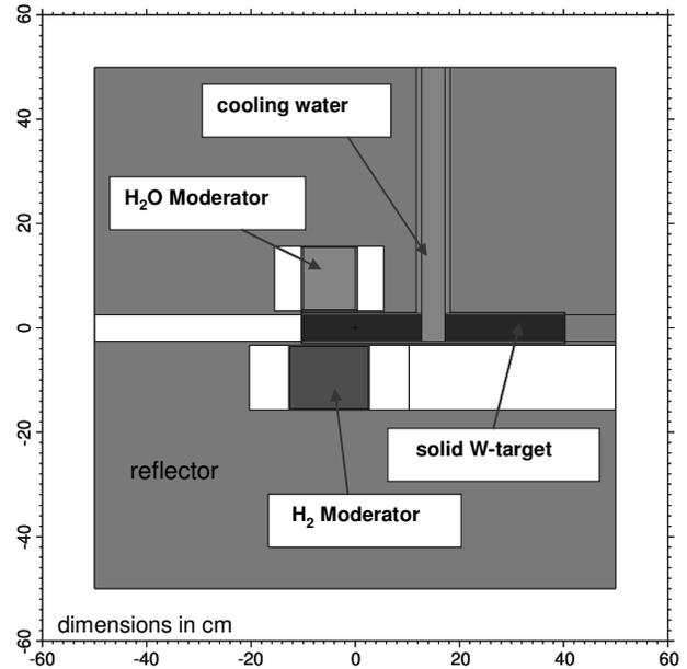
Fig. 2. Vertical cut through the geometry model used in MCNPX for simulating the energy deposition and neutron spectra. Dimensions are in cm.
