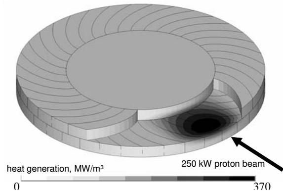
Fig. 6. Heat generation inside the segmented target for a 250 kW proton beam (pessimistically assumed to be 150 kW<sub>th</sub>) and an elliptical footprint with the two radii  $r_x = 10$  cm and  $r_y = 1.5$  cm. A parabolic intensity distribution within the footprint was assumed.
