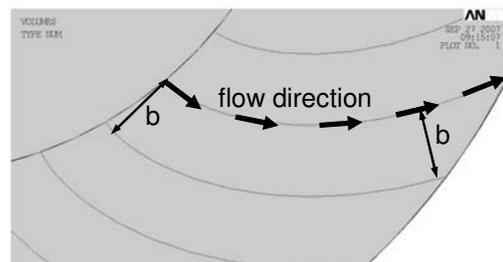
Fig. 7. Involute shaped segments have a constant thickness perpendicular to the flow direction.
