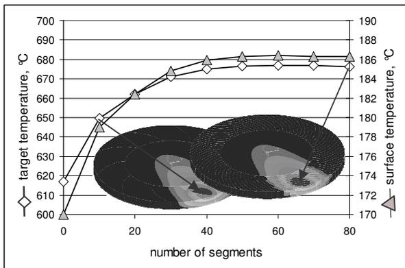
Fig. 11. Maximum temperature inside the target and at the cooled surface of the target as a function of the number of segments.
