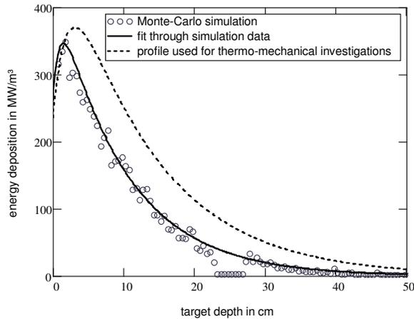
Fig. 4. Time averaged energy deposition along the proton beam axis.
