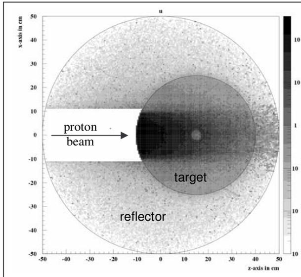
Fig. 3. Spatial distribution of the time averaged power deposited in the mid-plane of the tungsten target. The spot in the center of the target marks the cooling water tube. The energy deposition is given in  $\text{MW}/\text{m}^3$ .
