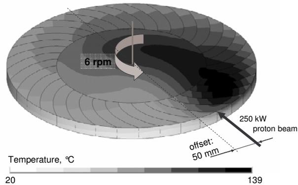
Fig. 13. Temperature distribution within a rotating segmented target. Due to the rotation a more even temperature distribution at low level is achieved.
