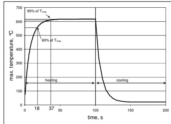
Fig. 10. Maximum temperature inside the target as a function of time for 100 s of heating-up and 100 s of cooling-down
