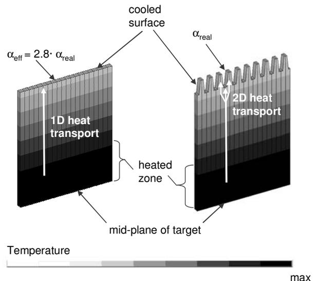
Fig. 8. A two-dimensional model was used to assess the heat transfer at the cooled surfaces of the segments. The effective heat transfer coefficient for the simplified flat surface (left side) was adjusted such that the same temperature distribution is achieved compared with the more detailed model (right side).
