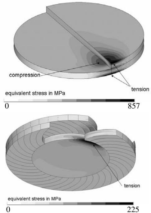
Fig. 12. Stress distribution within a monolithic solid target and within a segmented target. Due to the segmentation secondary stresses can be reduced significantly.
