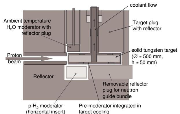
Fig. 1: Proposed target concept for the spallation neutron source in the Basque Country
