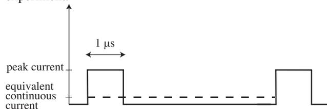
**Equivalence between pulsed current and continuous current.**
