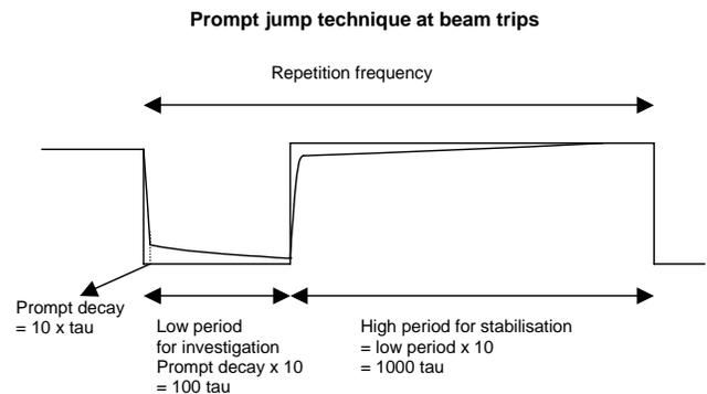
In a typical fast reactor the characteristic values are for  $L=1 \mu s$ ,  $\beta = 300 \text{ pcm}$  and  $\rho = -5000 \text{ pcm}$ , we obtain:  $\tau= 20 \mu s$ .
