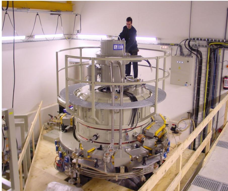
Fig. 2. 7 MeV, 700 kW IBA Rhodotron™ Electron Accelerator
