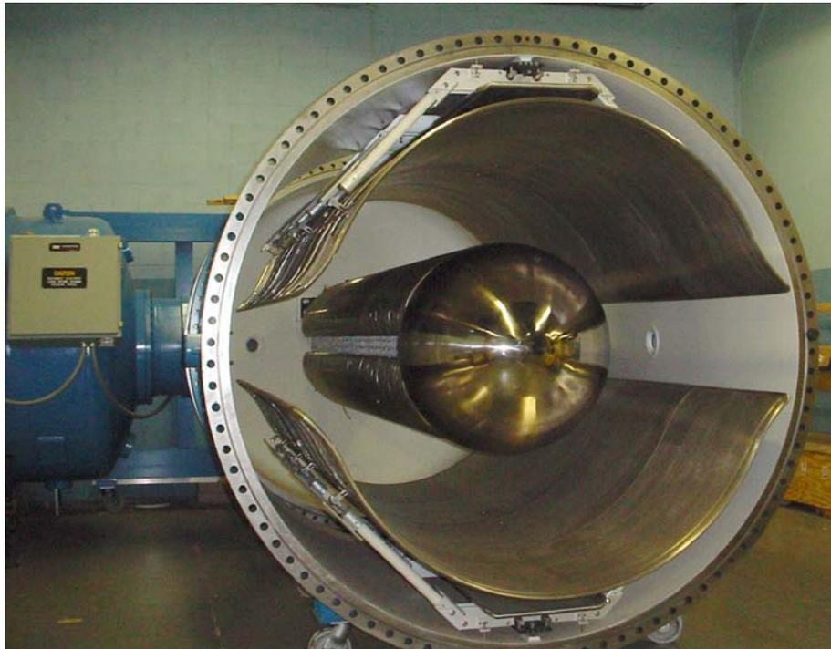
Fig. 1. 5 MeV, 300 kW RDI Dynamitron™ Electron Accelerator
