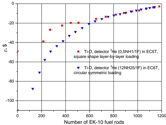
Fig.5. Reactivity versus number of EK-10 fuel rods with the PNS area method
