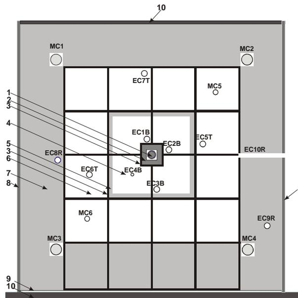
Fig. 2. X-Y cross section of the YALINA-Booster subcritical assembly
