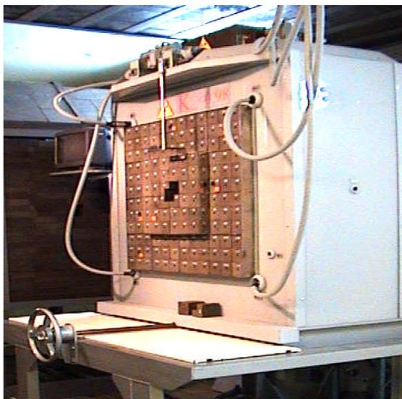
Fig.1. General view the YALINA-Booster subcritical assembly
