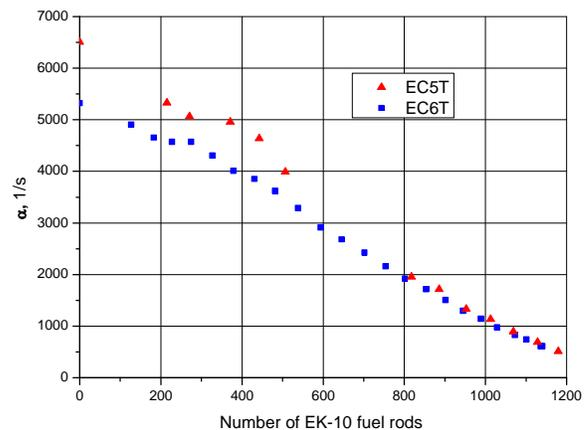
Fig.4. Prompt neutron flux decay constant ( $\alpha$ ) measured in the experimental channels EC5T and EC6T of the thermal zone using D-T neutrons in pulse mode
