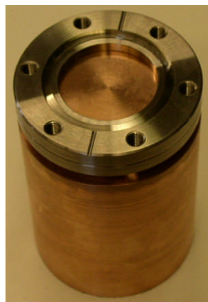
Figure 1. ISU RACE Target (the top piece is the conflate flange used to attach the target to the vacuum tube).
