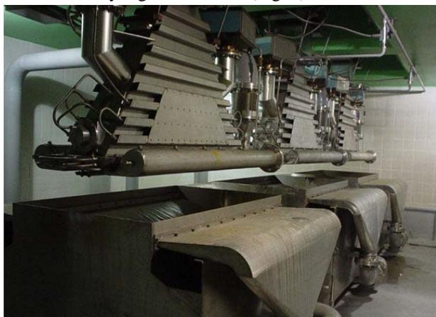
Fig. 3 High power accelerator in wastewater process
