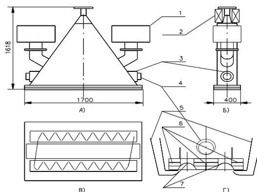
Fig. 2 Double extraction window: 1 ion pumps, 2 scanning system, 3 cylinder flange, 4 protection cylinders, 5 foil blower, 6 foil frame, 7-extraction foils.
