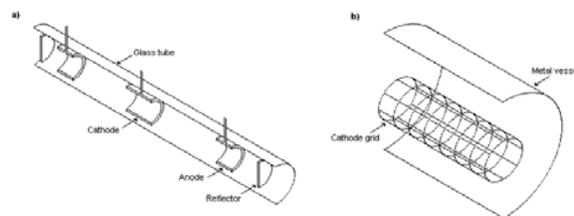
**Figure 2:** The two versions of the cylindrical IEC: a) axially-convergent ion beams, and b) radially-convergent ion beams (termed RC-IEC here).
