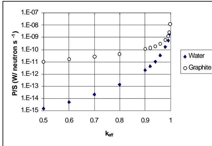
**Figure 4:** Power level per unit source (P/S) as a function as a function of  $k_{\infty}$  for two different moderators.
