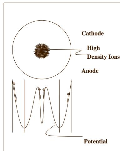
**Figure 1.** Illustration of the potential structure in the dense plasma core of a spherical IEC. The central "well" traps ions, providing efficient local ion re-circulation.
