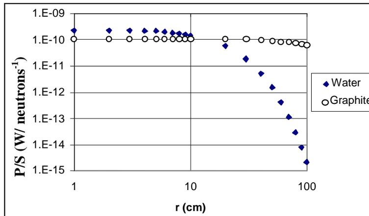
**Figure 5.** Power level per unit source as a function of the radius of the system for  $k_{\infty}=0.95$ . Notice that in the graphite-moderated system, P/S remains fairly constant for systems up to 50 cm in radius.
