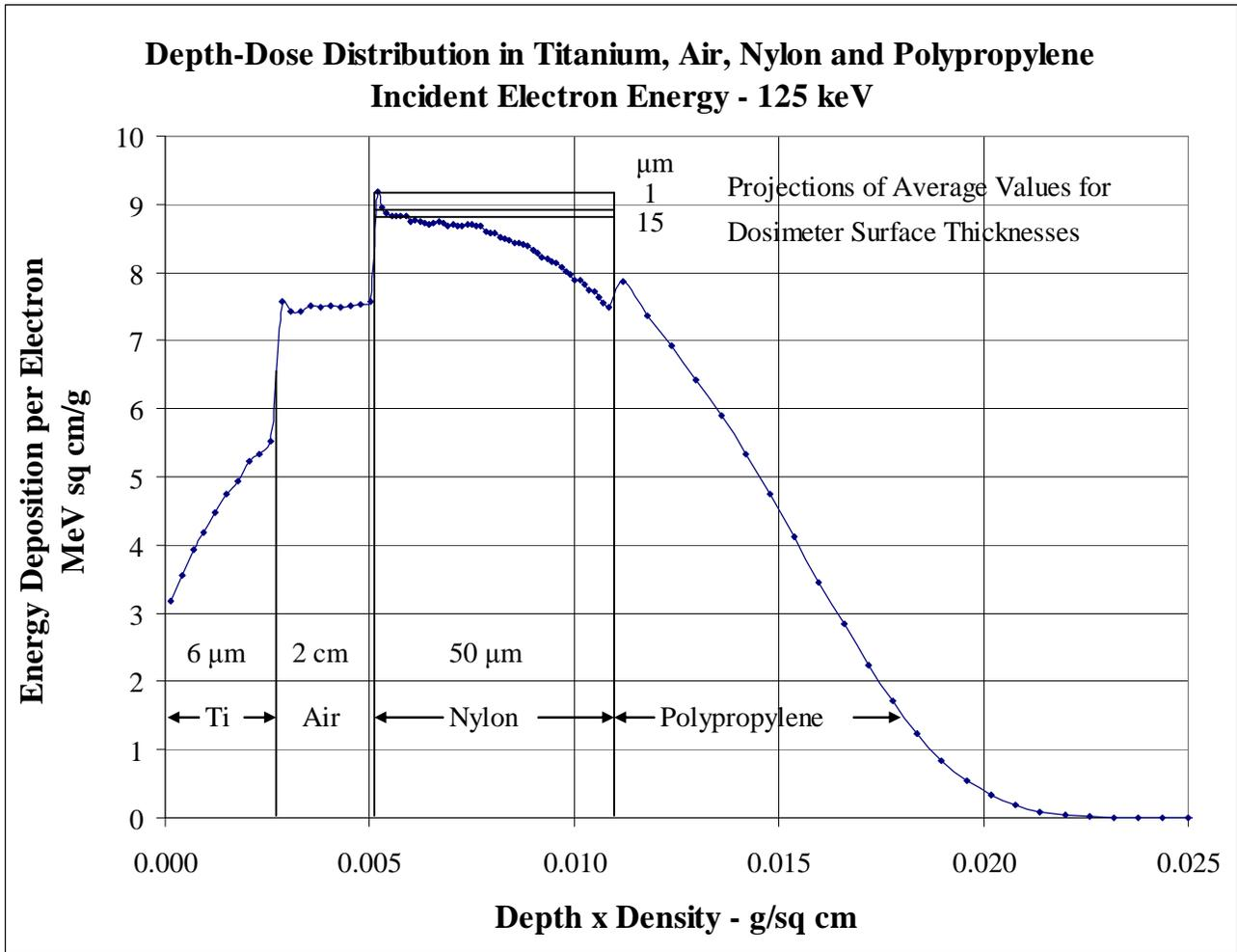
Fig.3. Energy deposition per electron vs depth x density in titanium, air, nylon and polypropylene at 125 keV.
