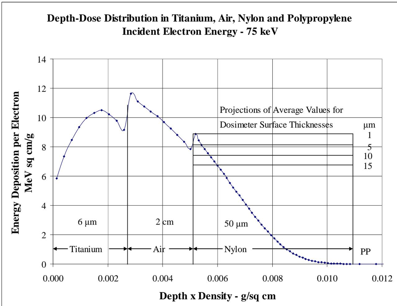
Fig.1. Energy deposition per electron vs depth x density in titanium, air, nylon and polypropylene at 75 keV.
