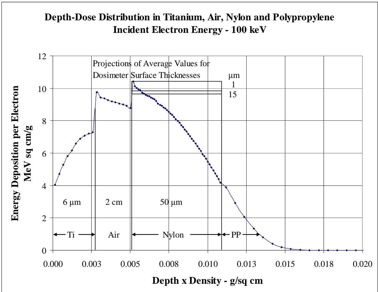
Fig. 2. Energy deposition per electron vs depth x density in titanium, air, nylon and polypropylene at 100 keV.
