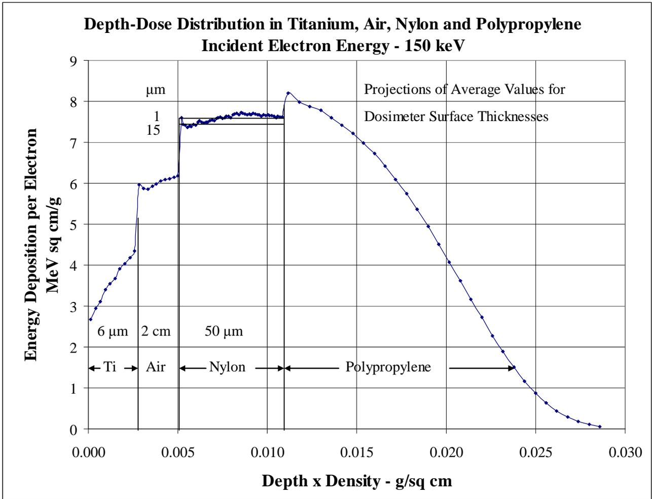
Fig. 4. Energy deposition per electron vs depth x density in titanium, air, nylon and polypropylene at 150 keV.
