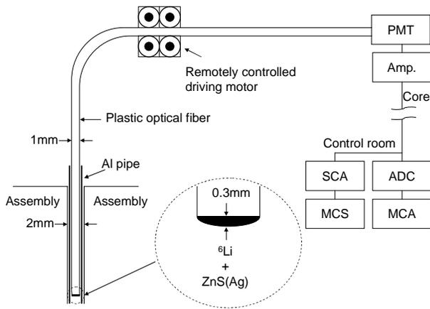
Fig. 3. Schematic view of the optical fiber detector system utilized in measurement of the neutron decay constant and subcriticality by the pulsed neutron method.
