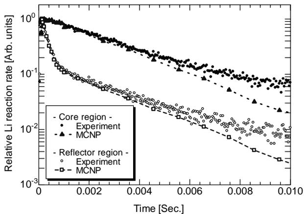
Fig. 4. Comparison of spatial dependence on neutron decay obtained by the optical fiber detector system set in both core and reflector regions.
