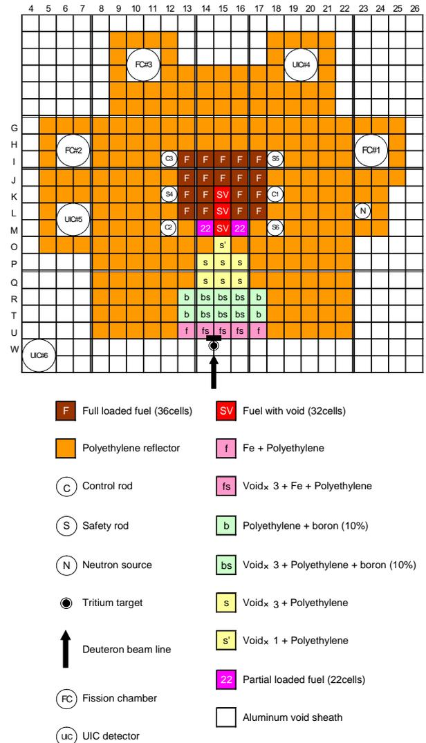
Fig. 1. Core configuration of ADSR experiments with 14MeV neutrons at KUCA A-core.
