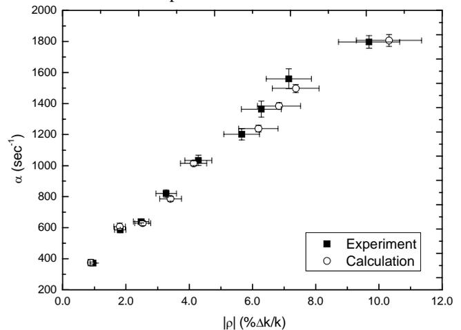
Fig. 5. Comparison of measured and calculated relation between subcriticality by the pulsed neutron method and neutron decay constant.
