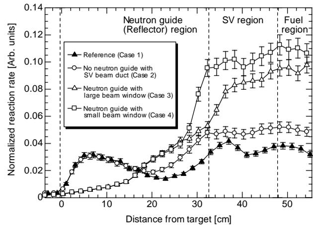
Fig. 2. Measured reaction rate distributions obtained from ADSR experiments with 14MeV neutrons.
