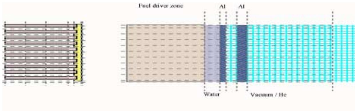
**Fig. 4** Examples of the HEADE models employed for the (a) LEU fuel assembly and (b) for the Neutron Guide System (SF) in beam tube L2 with the shielding tank filled with He.
