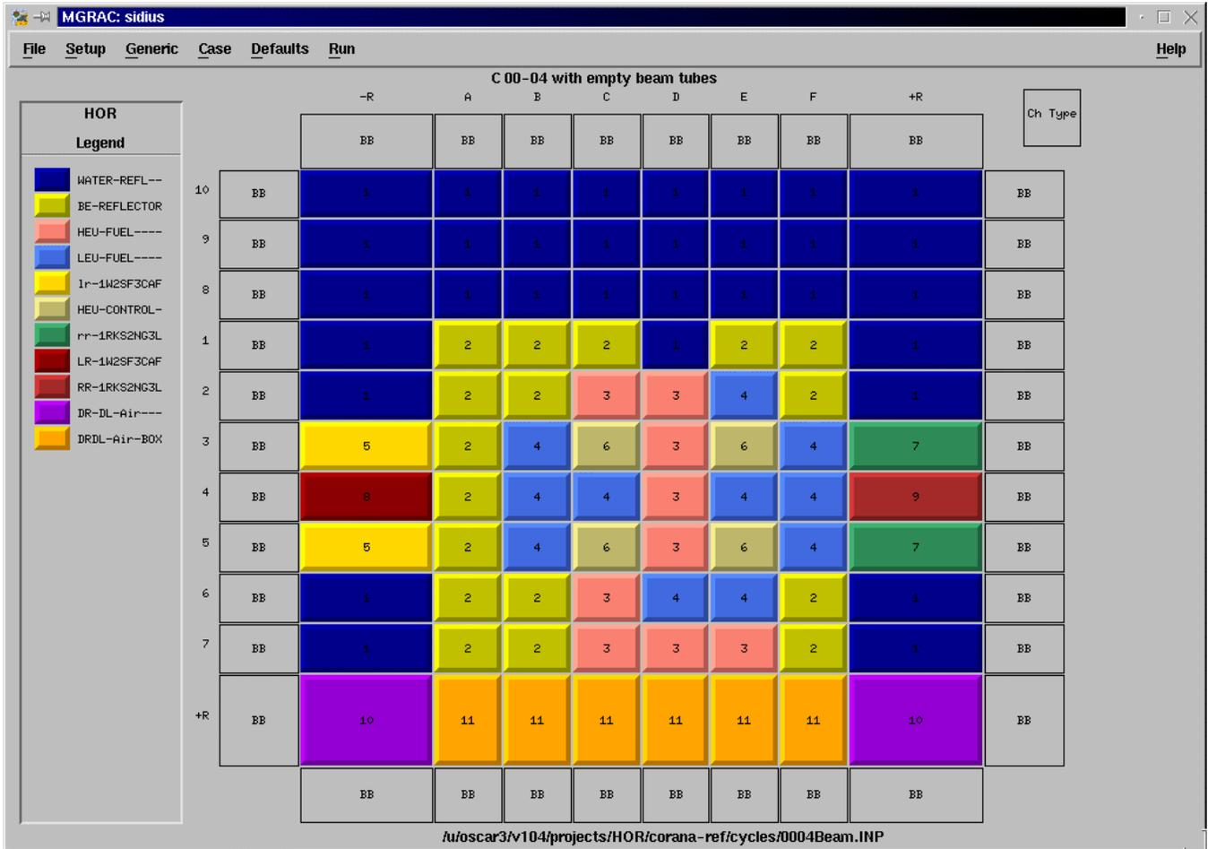
**Fig. 5** Cycle 0004 core load map as represented in MAESTRO. The reflector areas where beam tubes are modelled can clearly be distinguished from the water regions.
