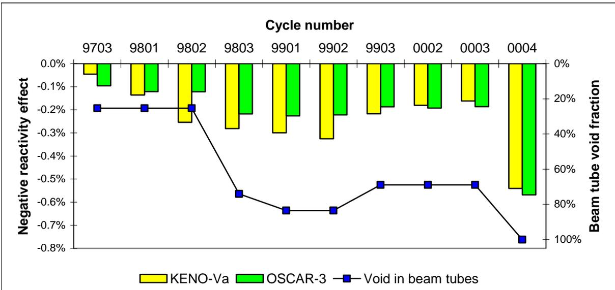
**Fig. 7** Relative Reactivity Effect of Empty Beam Tubes.
