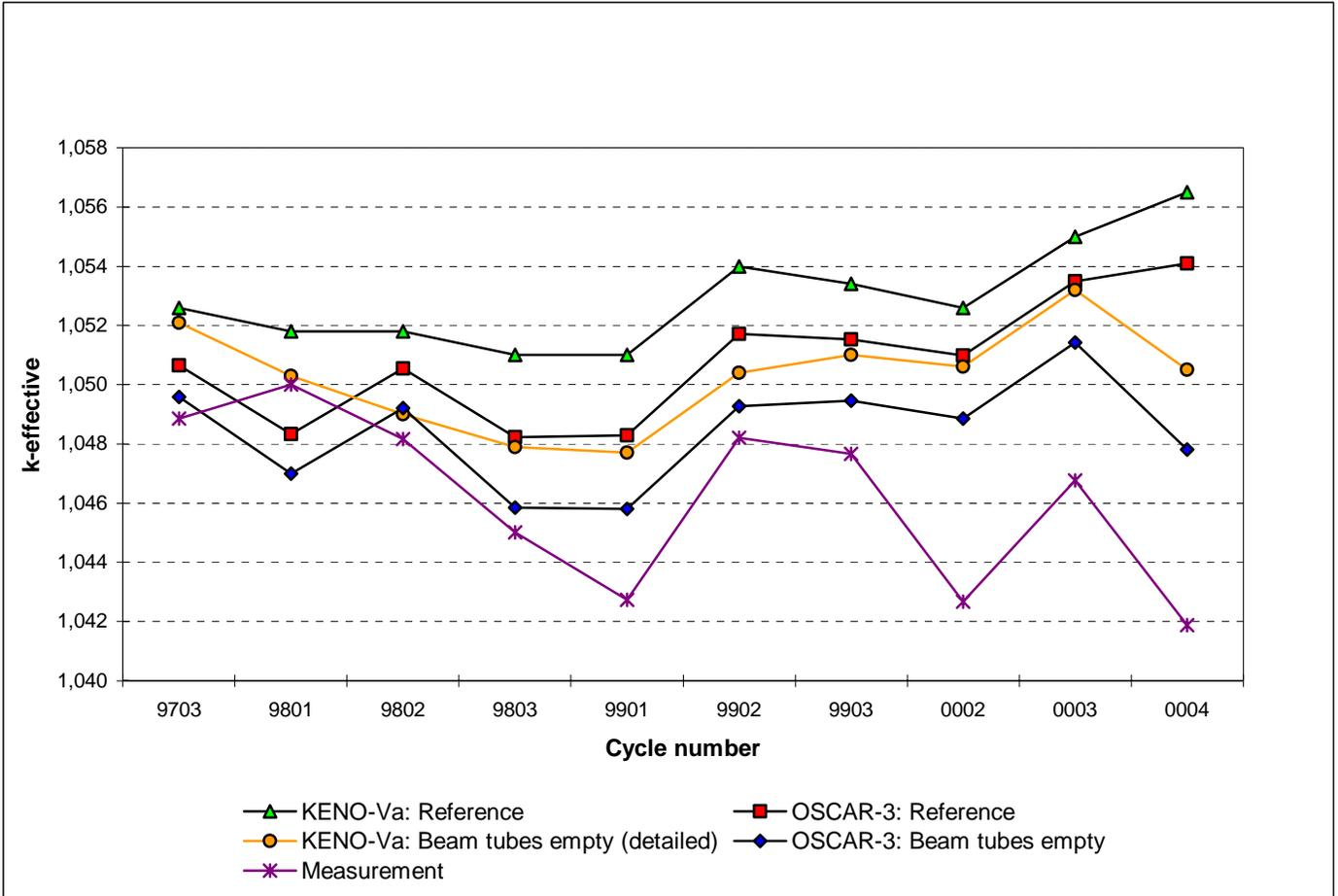
**Fig. 6** k-effective for different core cycles.
