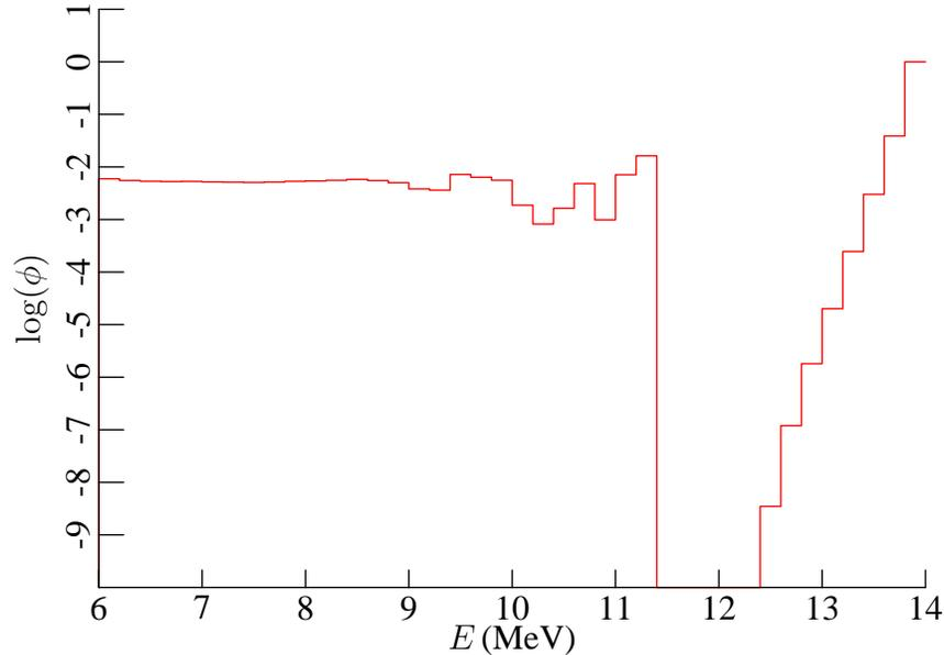
**Figure 1:** The neutron spectrum generated by 14 MeV neutrons slowing down in Pb-208; computed using  $2 \times 10^8$  particles in MCNP. Note the large flux depression just below the source energy.
