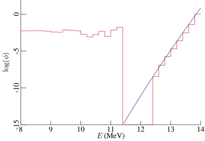
**Figure 2:** The neutron spectrum near the source energy, generated by 14 MeV neutrons slowing down in Pb-208. Red line: computed using  $2 \times 10^8$  particles in MCNP. Blue line: computed from Eq. 8 with  $K = 0.0056$ . Recall that in those regions of phase space where the Monte Carlo results are absent there were *no* simulation particles.
