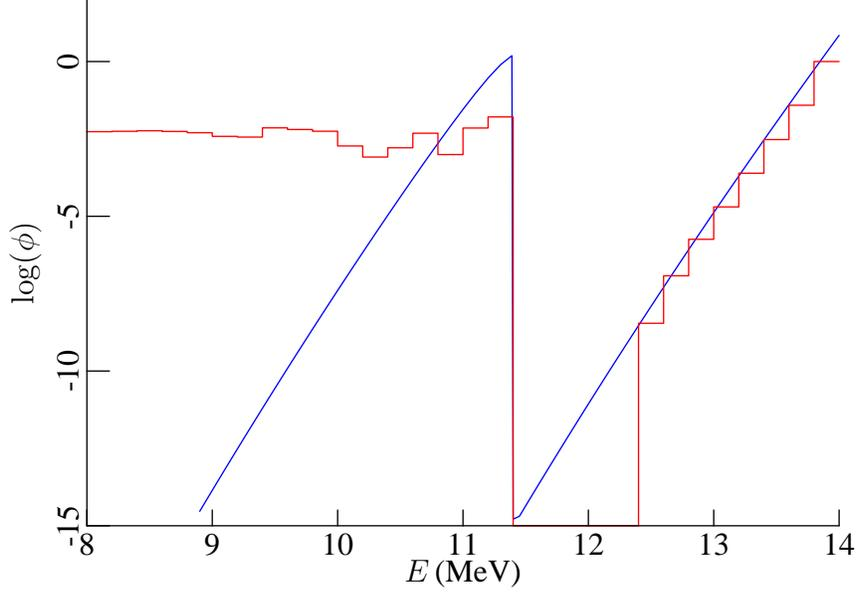
**Figure 3:** The neutron spectrum near the source energy, generated by 14 MeV neutrons slowing down in Pb-208. Red line: computed using  $2 \times 10^8$  particles in MCNP. Blue line: computed from the simple model with  $K = 0.0056$  and  $p = 0.2957$ . Note that the modeled flux (blue) is not discontinuous at 11.4 MeV, but it does change very rapidly there.
