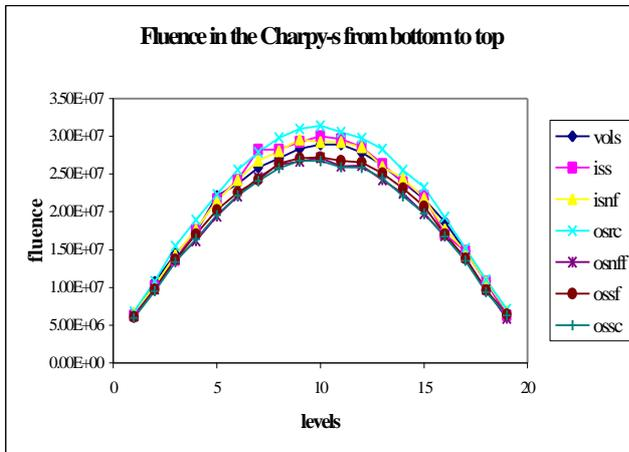
Fig.5.1. The fluence calculated in the Charpy-s
