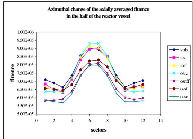
Fig.5.7. Azimuthal change of the axially averaged fluence in the half of the reactor vessel.
