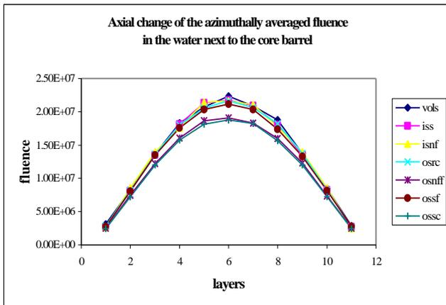
Fig.5.4. Axial change of the azimuthally averaged fluence in the water next to the barrel.
