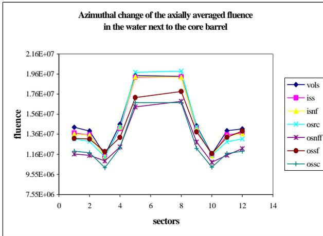
Fig.5.6. Azimuthal change of the axially averaged fluence in the water next to the barrel.
