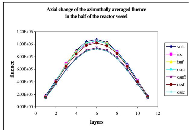
Fig.5.5. Axial change of the azimuthally averaged fluence in the half of the reactor.
