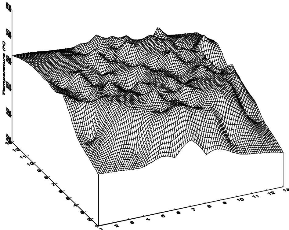
Figure 7 Nodal Temperature Distribution at 35 sec
