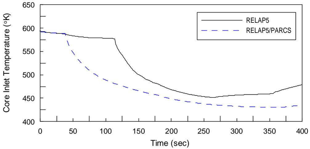
Figure 4 Core Inlet Temperature in LOOP A
