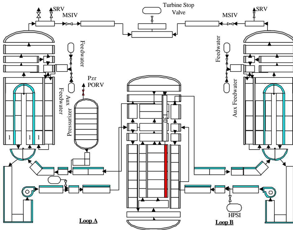
Figure 2 RELAP5 System Nodalization
