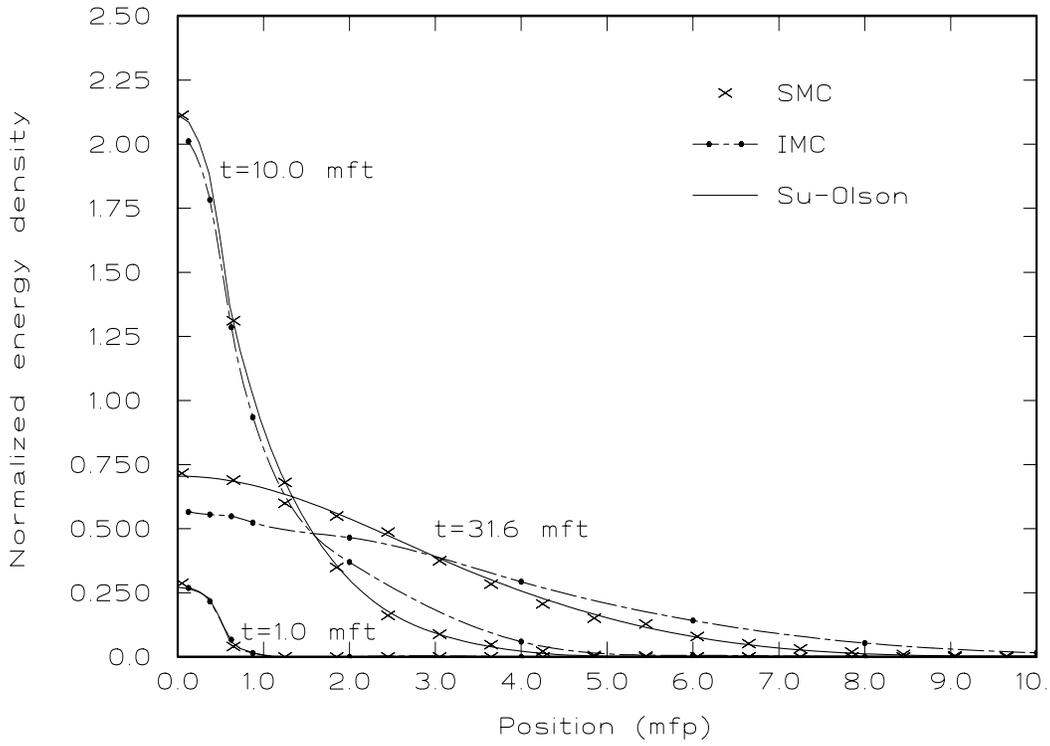
**Fig 2:** Material Energy Density ( $\alpha = 0.5$ , coarse  $\Delta z$ , fine  $\Delta t$ )
