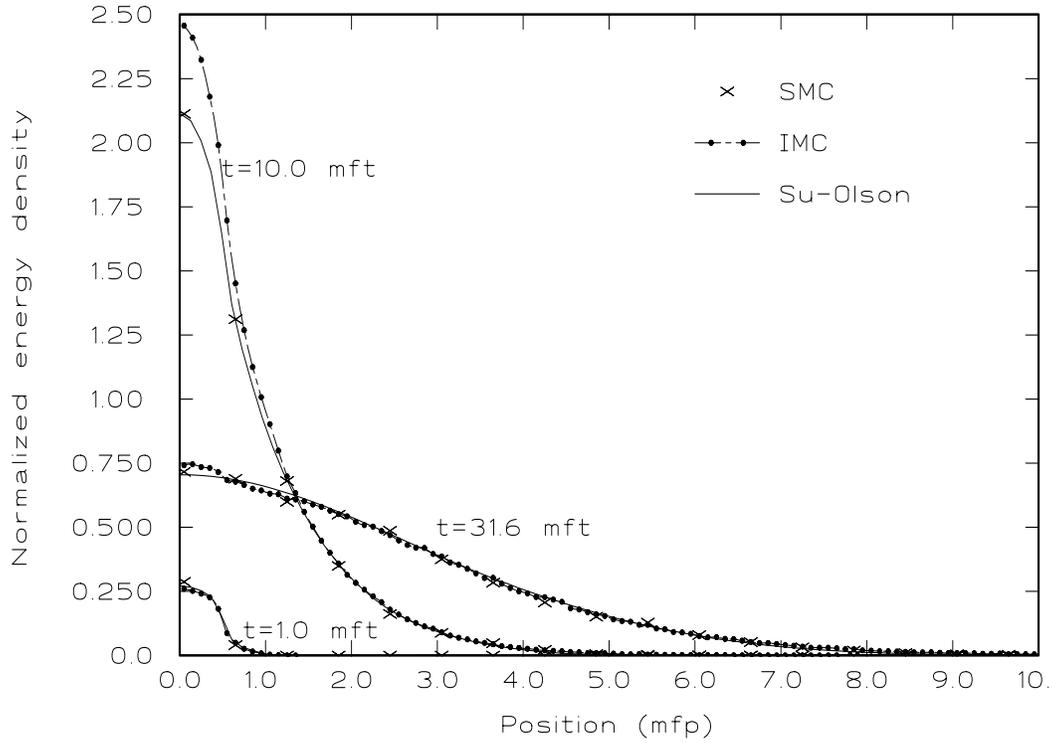
**Fig 3:** Material Energy Density ( $\alpha = 0.5$ , fine  $\Delta z$ , coarse  $\Delta t$ )
