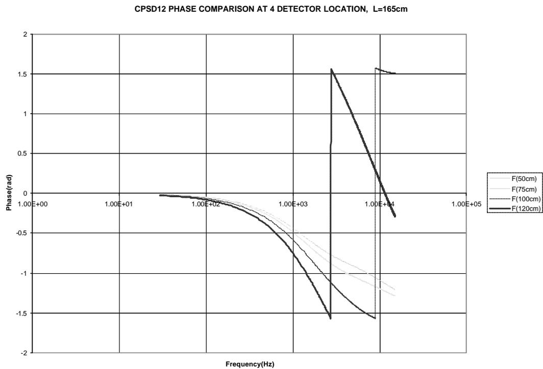
Figure 8. CPSD<sub>12</sub> theoretical phase comparison at 4 detector locations.
