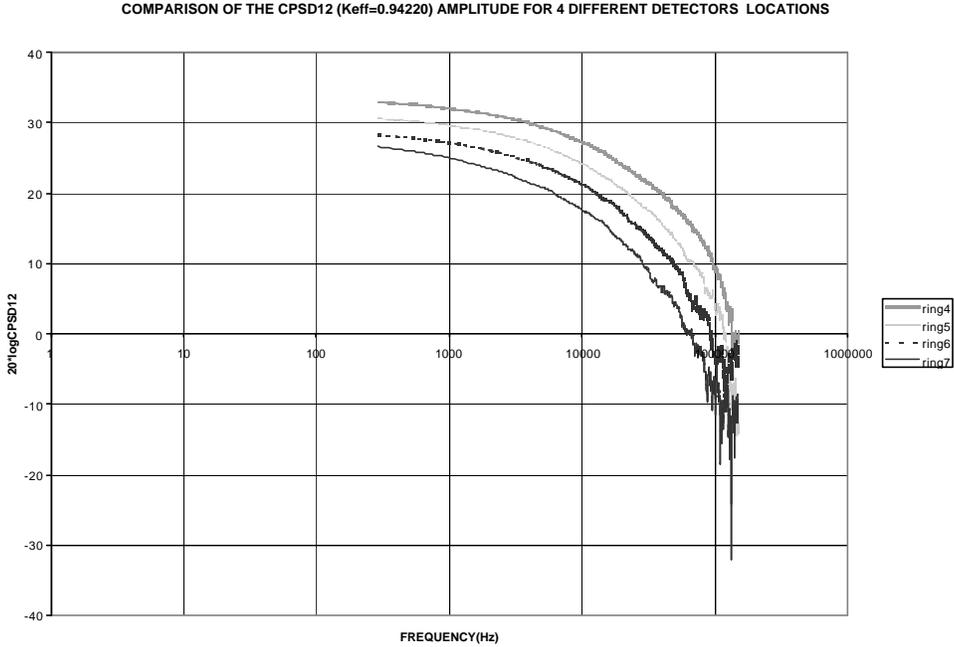
Figure 2. Amplitude of the source-detector CPSD.
