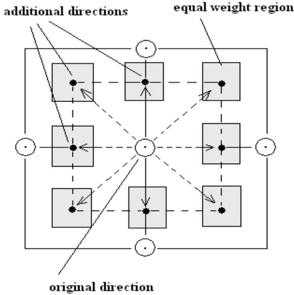
**Fig. 5** Ordinate Splitting Technique
