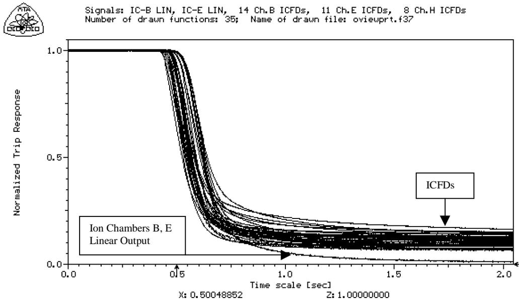
Figure 15. Normalized signals of ICFDs and ion chambers used in reactor regulating and shutdown systems responding to an SDS2 trip from 60% full power in Pickering-B Unit 6 (new ICFDs)
