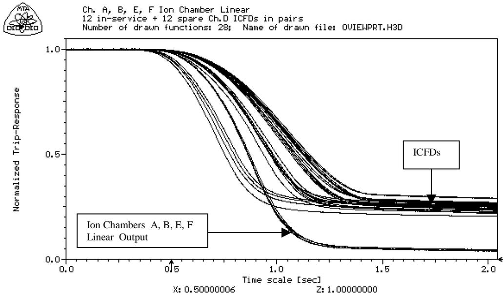
Figure 14. Normalized signals of ICFDs and ion chambers used in reactor regulating and shutdown systems responding to an SDS1 trip from 60% full power in Pickering-B Unit 8 (old ICFDs)
