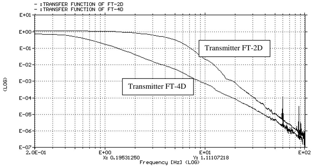
Figure 3. Magnitude of the dynamic transfer functions of Rosemount flow transmitters derived from in-situ pressure sensor noise measurements in shutdown system flow loops FT-2D and FT-4D in Pickering-B Unit 6
