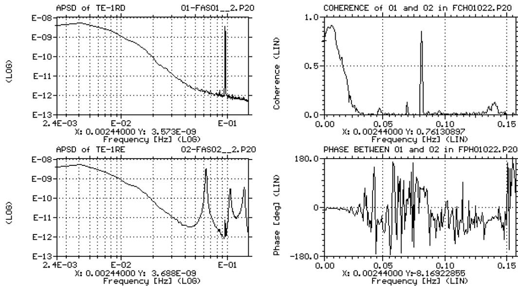
Figure 8. APSD, coherence and phase functions of moderator temperature fluctuations measured by two SDS1 strap-on RTDs located at reactor core outlet
