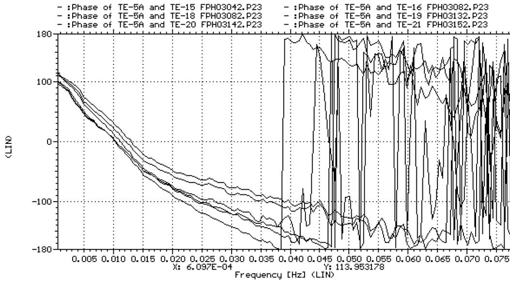
Figure 13. Phase functions between moderator temperature fluctuations measured by a core outlet RTD and six other RTDs located at core inlet. The noise-based estimates of transit times varied with distance between RTDs, and were between 6.9 and 13.0 sec
