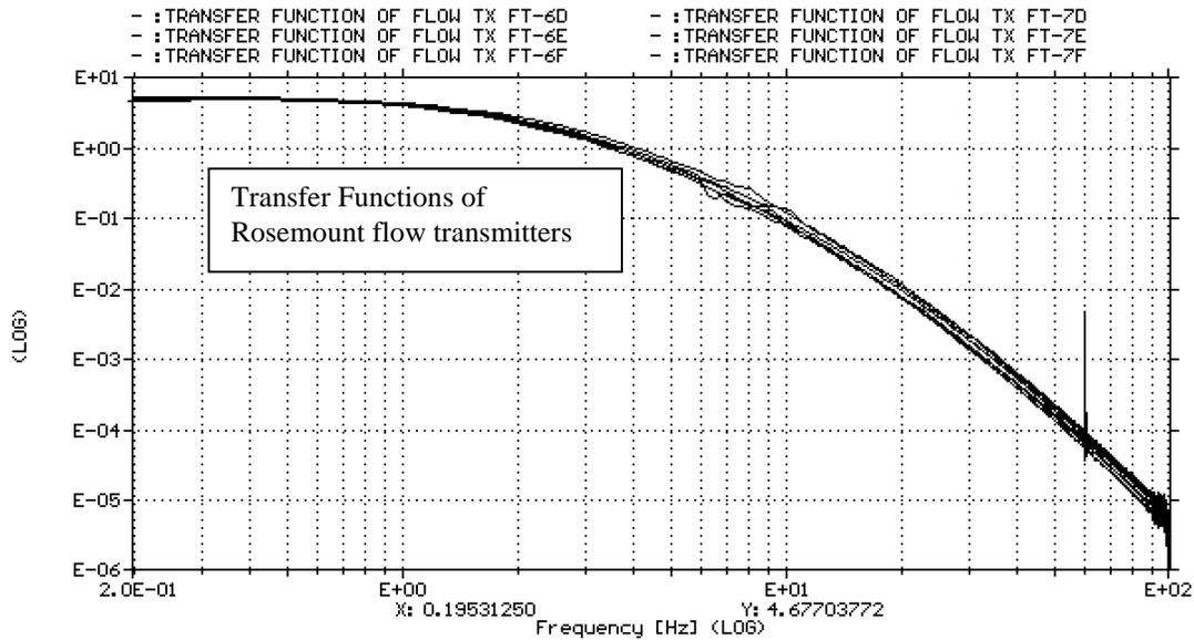
Figure 2. Magnitude of the dynamic transfer functions of Rosemount flow transmitters derived from in-situ pressure noise measurements in SDS1 flow loops in Bruce-B Unit 6
