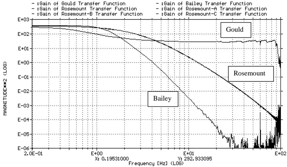
Figure 1. Magnitude of the dynamic transfer functions of Rosemount, Gould, and Bailey flow transmitters, derived from in-situ pressure sensor noise measurements in shutdown system flow loop FT-3J in Darlington Unit 3
