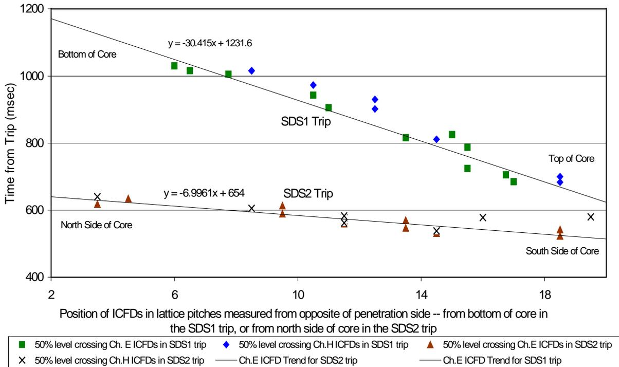
Figure 16. Comparing the 50% level crossing times of ICFD signals as a function of detector position, measured in SDS1 (1996) and SDS2 (2001) trips from 60% full power in Pickering-B Unit 6
