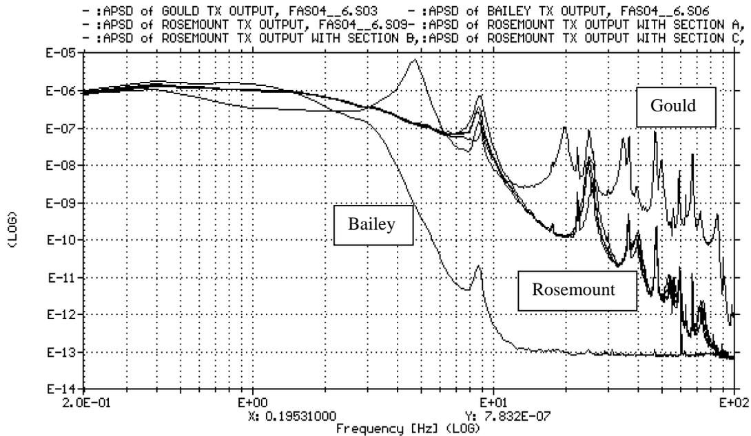
Figure 4. Comparing the normalized APSD functions of output flow noise signals of Rosemount, Gould, and Bailey flow transmitters installed on shutdown system flow loop FT-3J in Darlington Unit 3
