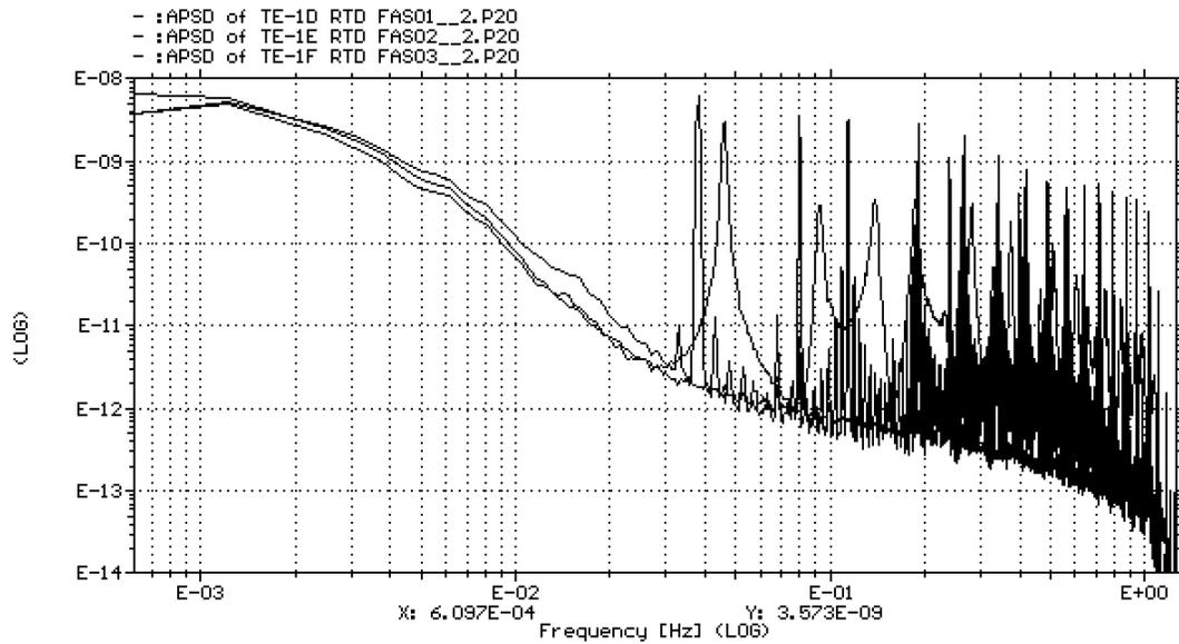
Figure 7. APSD spectra of moderator temperature fluctuations measured by three SDS1 strap-on RTDs located at core outlet in Bruce Unit 8. The noise-based response time estimates were between 60-100 sec
