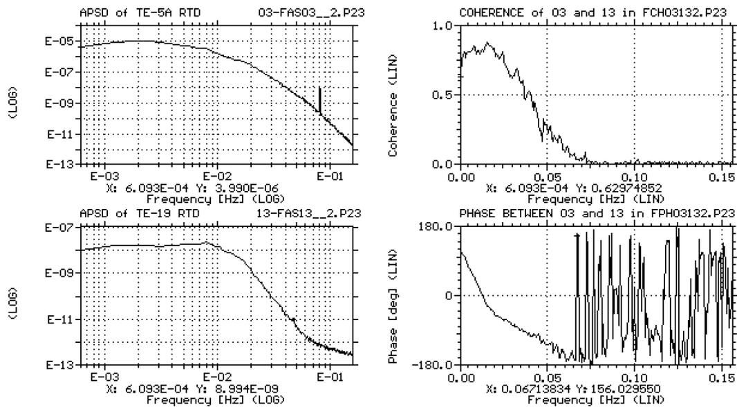
Figure 12. APSD, coherence and phase functions of moderator temperature fluctuations measured by two Reactor Regulating System thermal-well RTDs. One located at core outlet, the other at core inlet of moderator loop No.1
