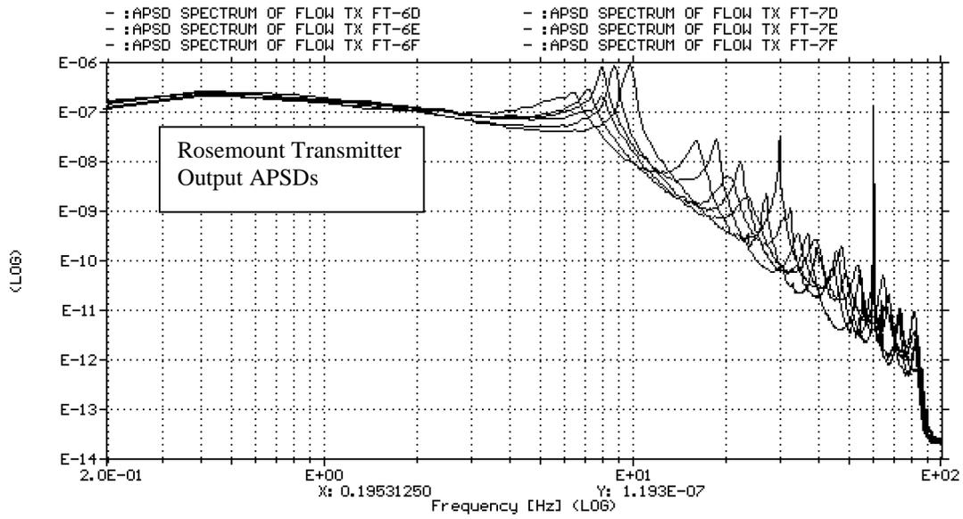
Figure 5. APSD spectral functions of the output noise signals of the six SDS1 Rosemount flow transmitters measured in Bruce-B Unit 6 at full power
