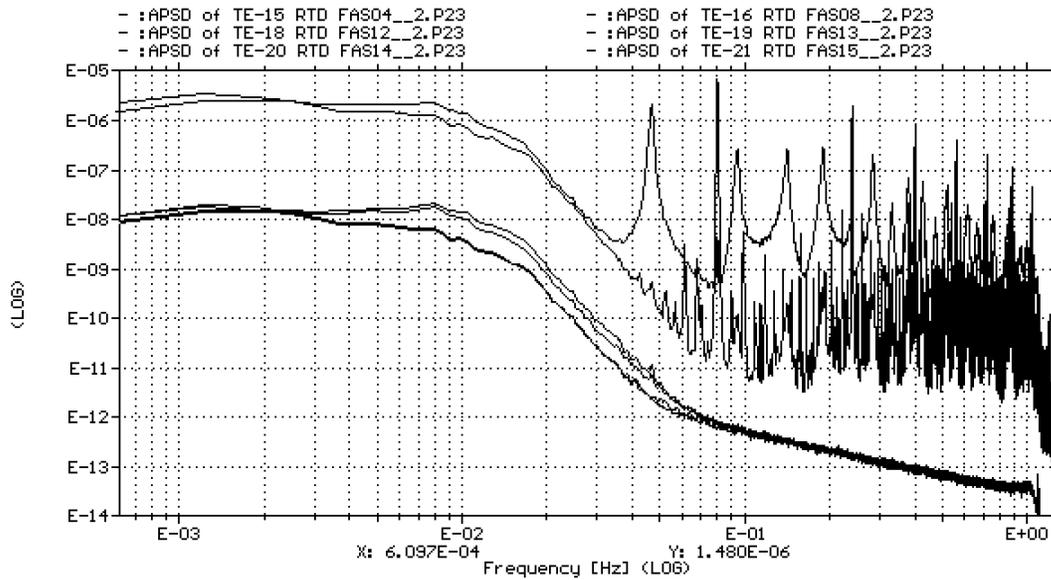
Figure 10. APSD spectra of moderator temperature fluctuations measured by six Reactor Regulating System thermal-well RTDs located at core inlet in Bruce Unit 8. The noise-based response time estimates were between 12-22 sec
