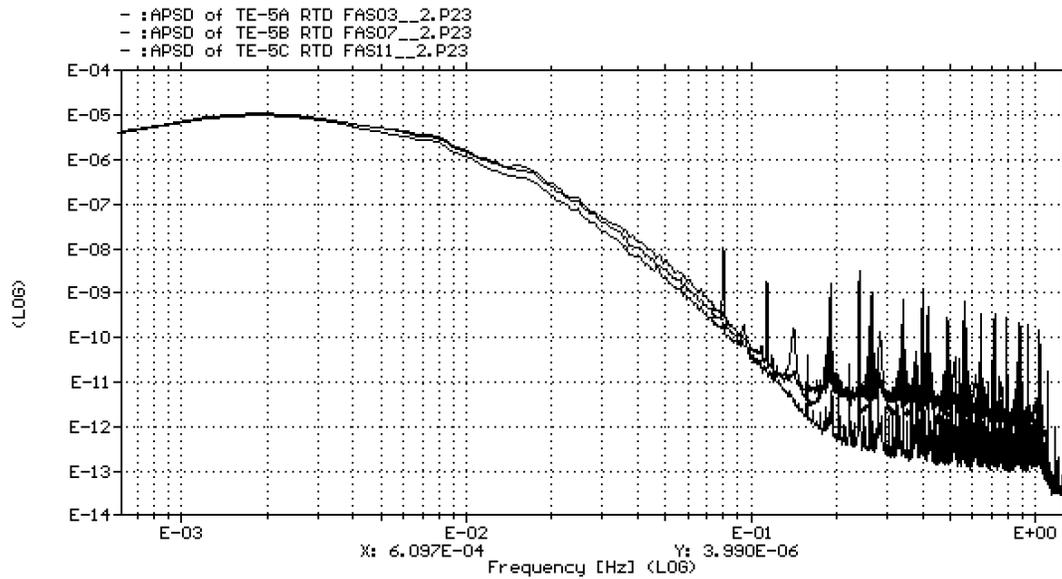
Figure 9. APSD spectra of moderator temperature fluctuations measured by three Reactor Regulating System thermal-well RTDs located at core outlet in Bruce Unit 8. The noise-based response time estimates were between 31 and 45 sec
