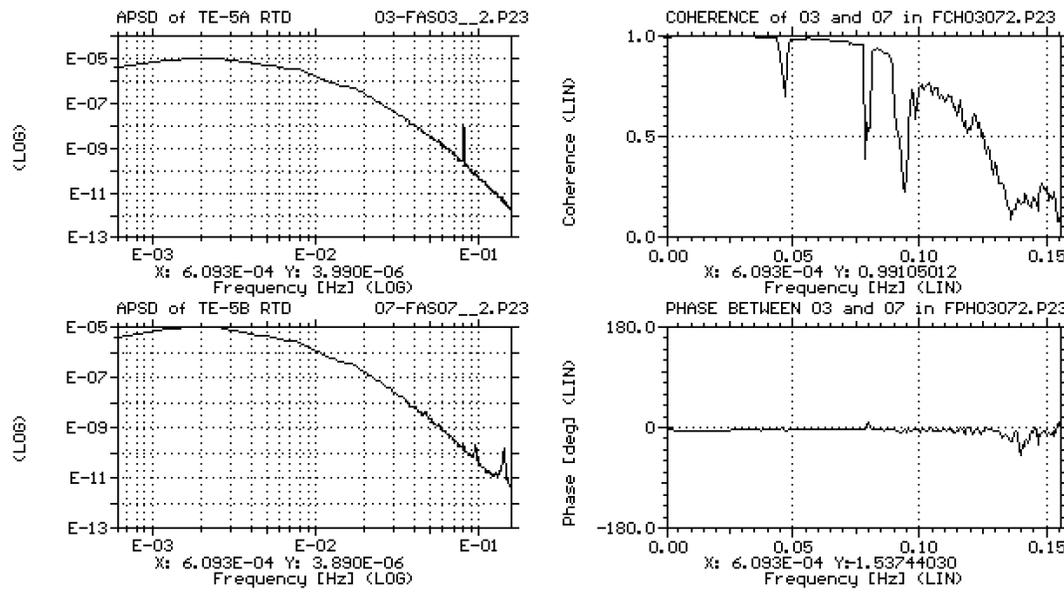
Figure 11. APSD, coherence and phase functions of moderator temperature fluctuations measured by two Reactor Regulating System thermal-well RTDs located at core outlet. The RTDs were in close proximity
