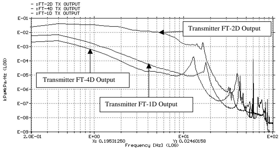
Figure 6. Comparing the APSD functions of output noise signals of Rosemount flow transmitters installed on shutdown system flow loops FT-1D and FT-4D with increased response time (500 msec), and FT-2D with shorter response time (less than 200 msec) in Pickering-B Unit 6
