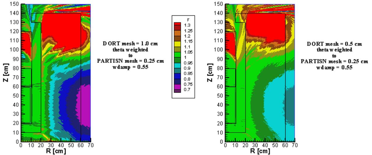
Figure 7. Ratio of DORT TW solutions for 1.0 and 0.5 cm mesh intervals to base case.
