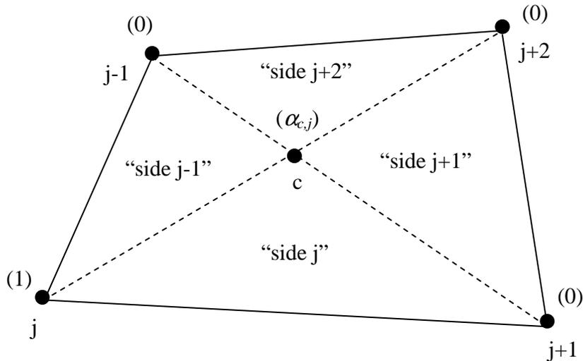
**Figure 3. Illustration of a quadrilateral cell  $c$ . The values of the basis function  $b_{c,j}(x,y)$  at vertices and the point  $c$  are shown in parentheses.**
