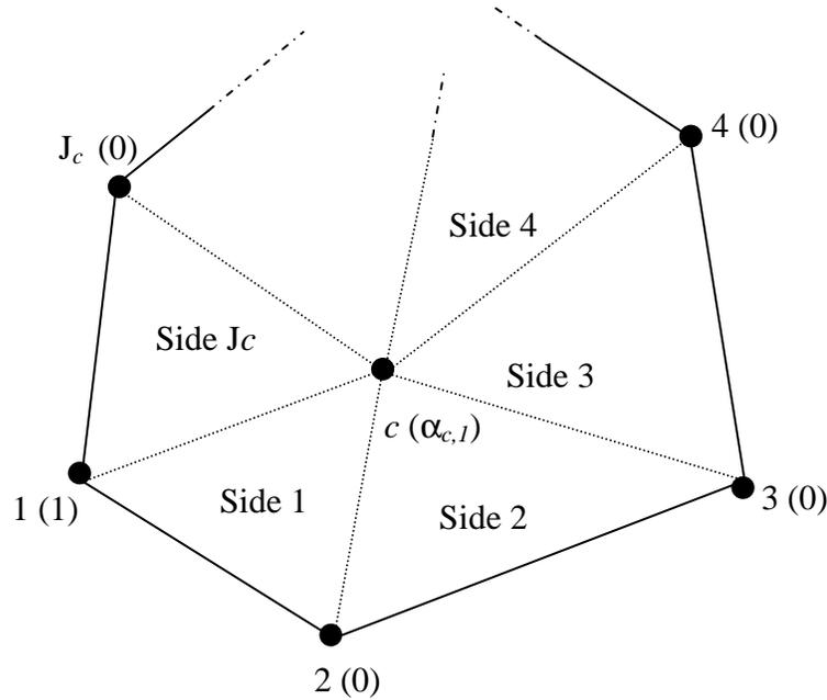
**Figure 4. Illustration of an arbitrary polygonal cell  $c$ . The values of the basis function  $b_{c,1}(x,y)$  at vertices and the point  $c$  are shown in parentheses.**
