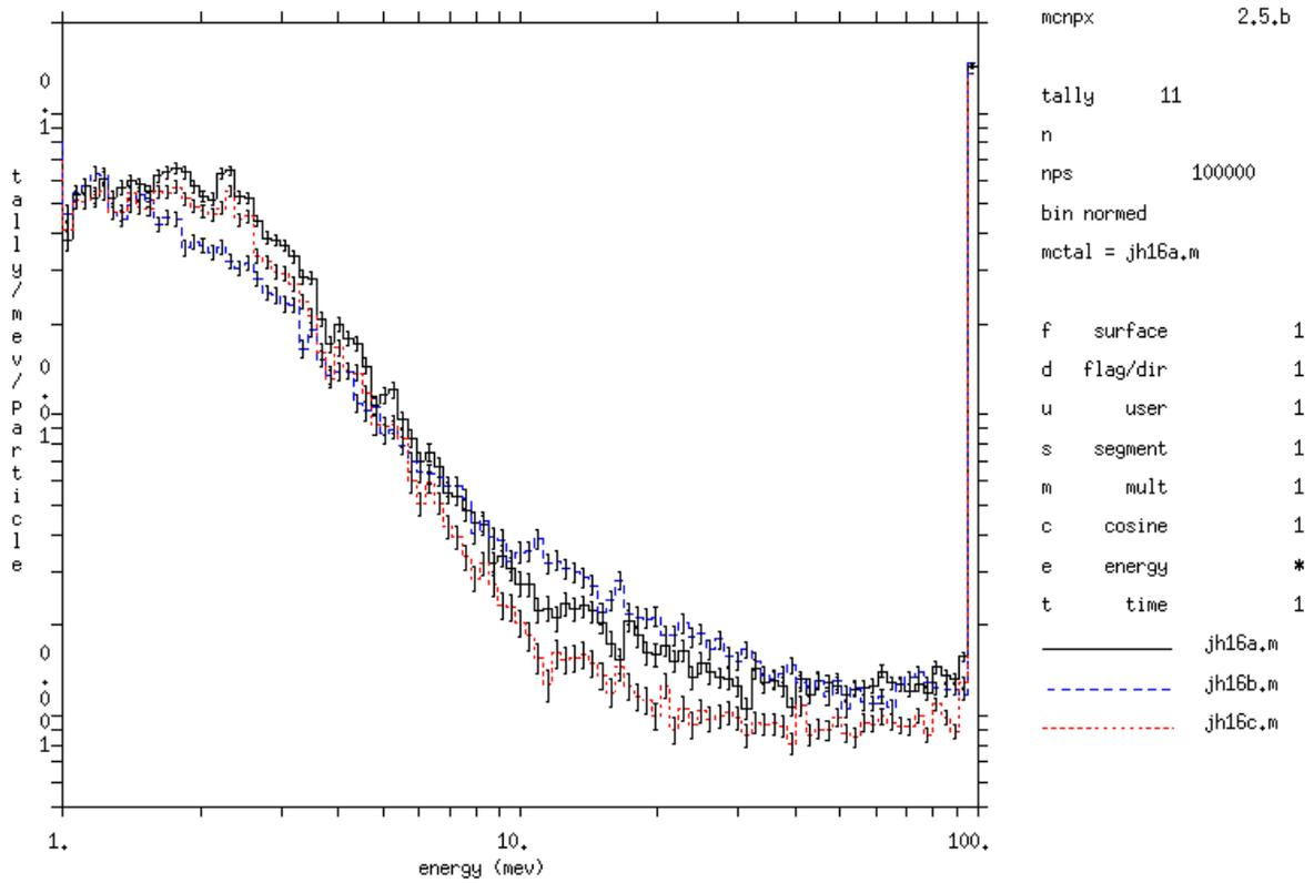
**Figure 2. Neutron Current Escaping Top of BGO Can**
