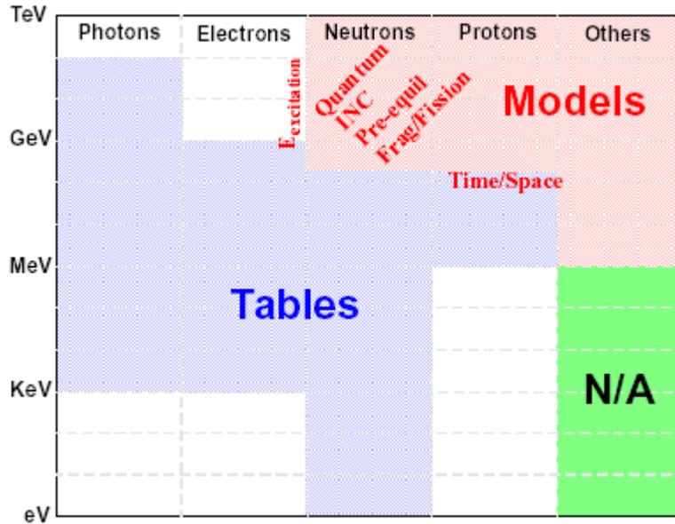
Figure 1. MCNPX PARTICLE ENERGY RANGES
