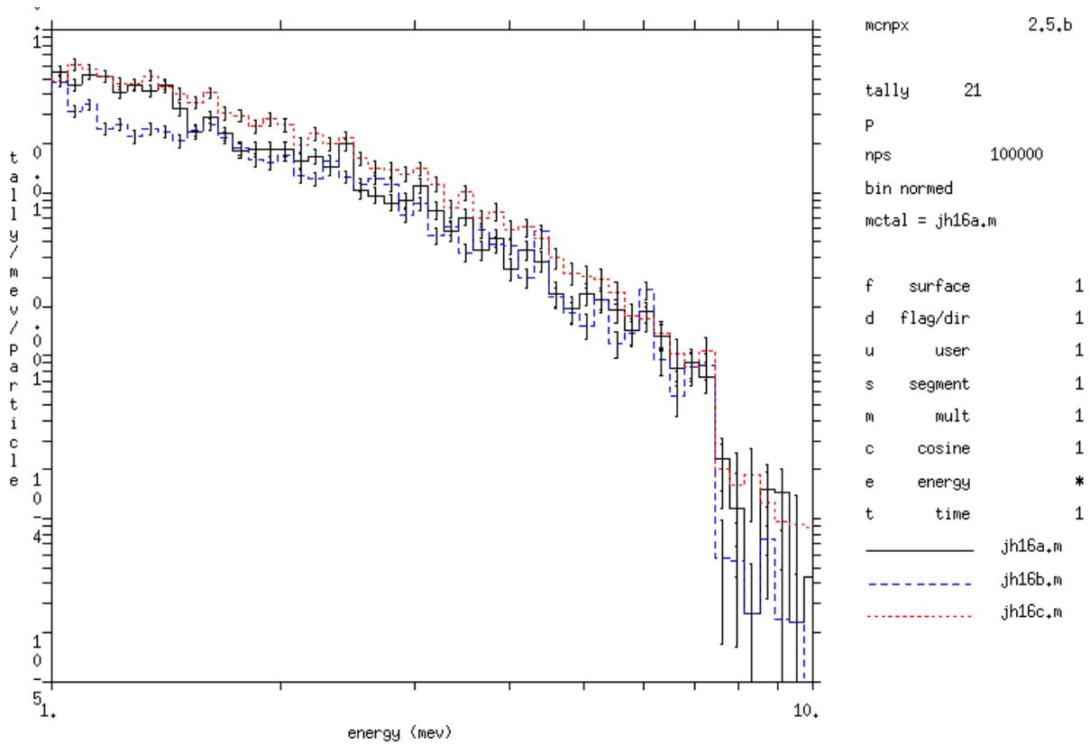
**Figure 3. Photon Current Escaping Top of BGO Can**
