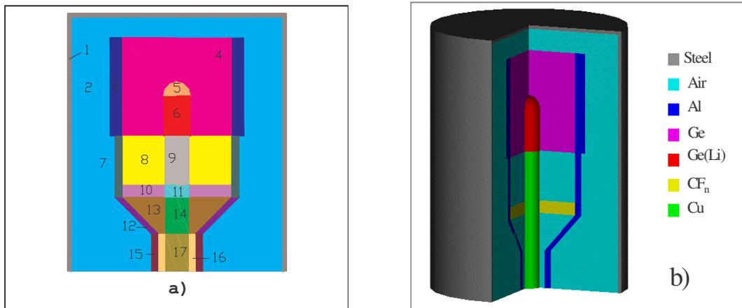
**Figure 3. A semiconductor detector geometry example: a) division into regions (frontal projection); b) material composition.**
