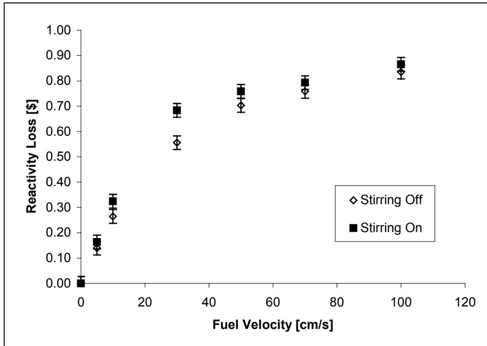
Figure 3. Reactivity loss with and without stirring the fuel at  $T_c=5$  s
