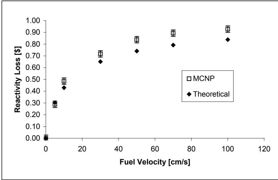
Figure 1. Calculated reactivity loss with recirculation time  $T_c = 100000$  s
