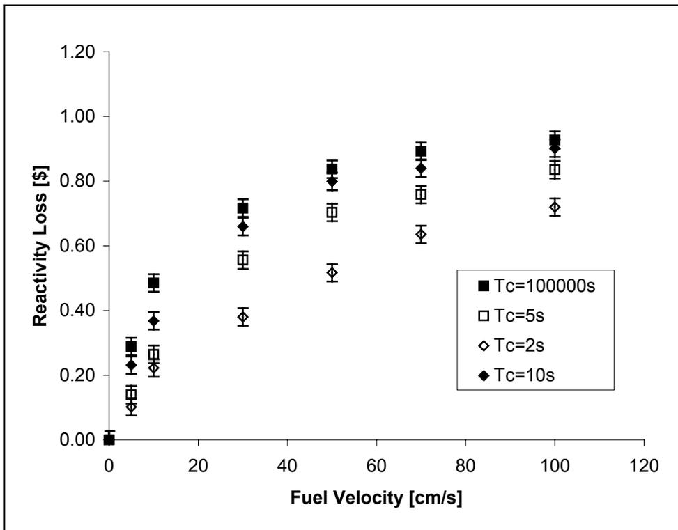
Figure 2. Reactivity loss as a function of fuel velocity and recirculation time
