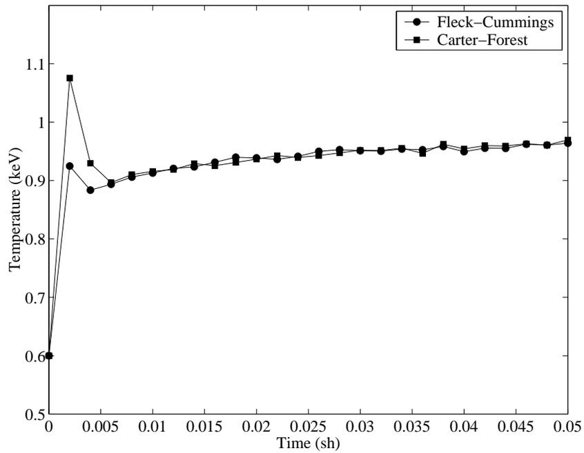
Figure 5. Material Temperature at  $x=\Delta x/2=0.05$  cm ( $T_i=0.6$  keV)
