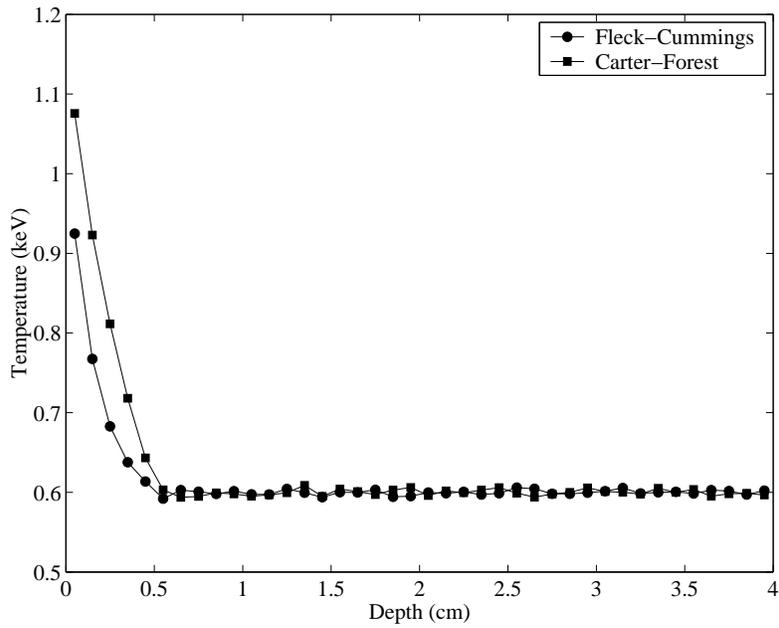
Figure 4. Material Temperature at  $t=\Delta t=0.002$  sh ( $T_i=0.6$  keV)
