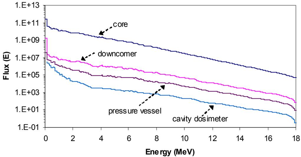
Figure 6. The 180-group flux spectra in the core, downcomer, pressure vessel and cavity dosimeter regions.
