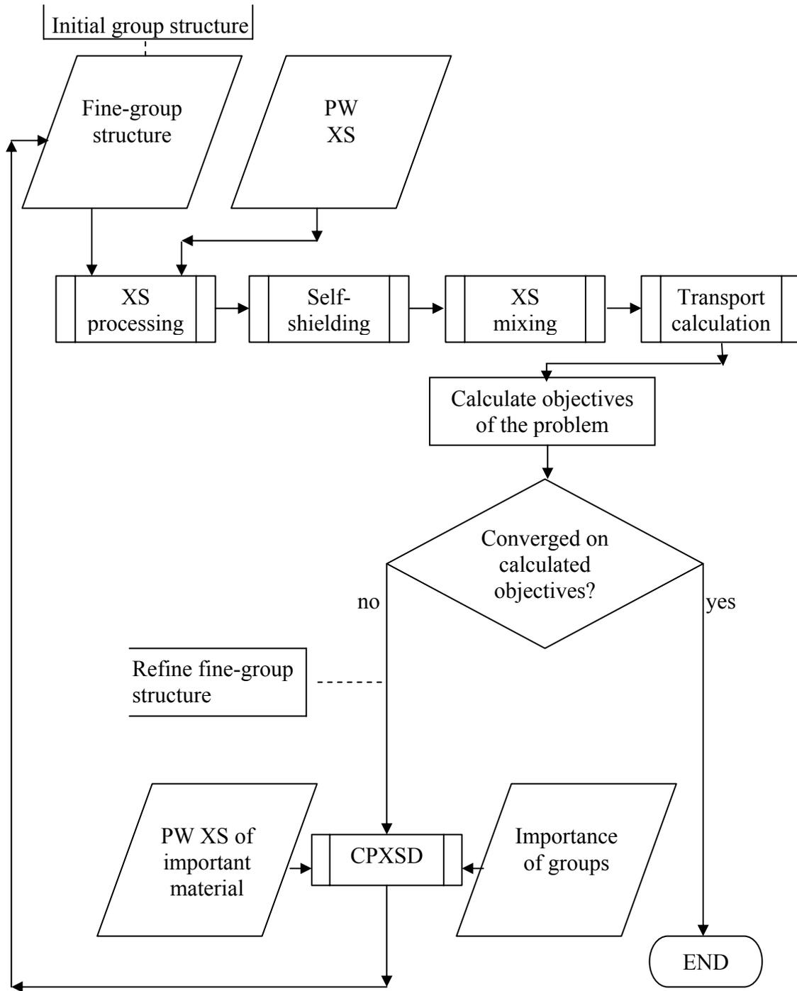
**Figure 2. Process for fine-group structure construction using the CPXSD methodology (XS and PW refer to cross-section and point-wise, respectively).**
