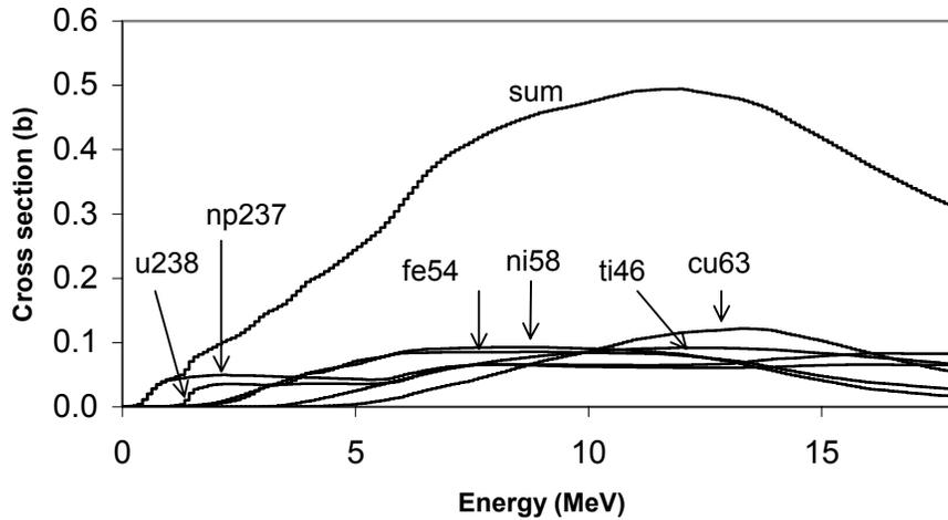
**Figure 4. Normalized dosimetry cross sections and their sum.**
