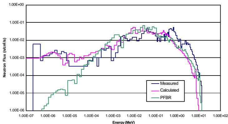
Figure 4. Comparison of Measured and Calculated Neutron Spectrum with PFBR Blanket Exit Spectrum
