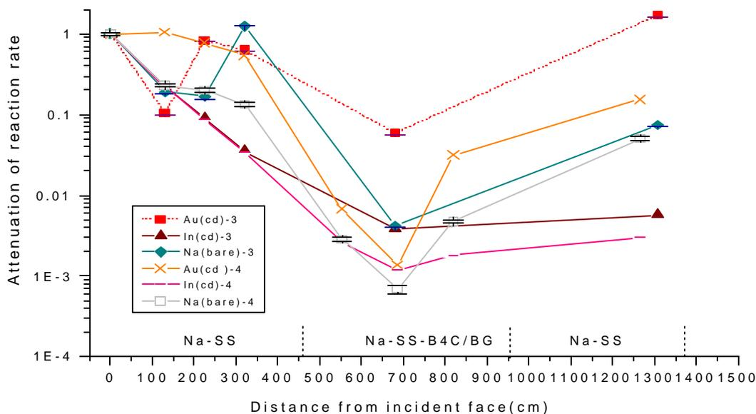
**Figure 6. Attenuation in Steel-Borated graphite/Boron Carbide-sodium Shields**
