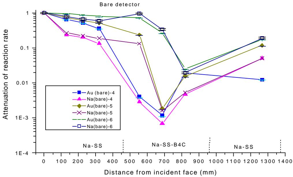
**Figure 8. Attenuation of Bare Foil Reaction Rates**
