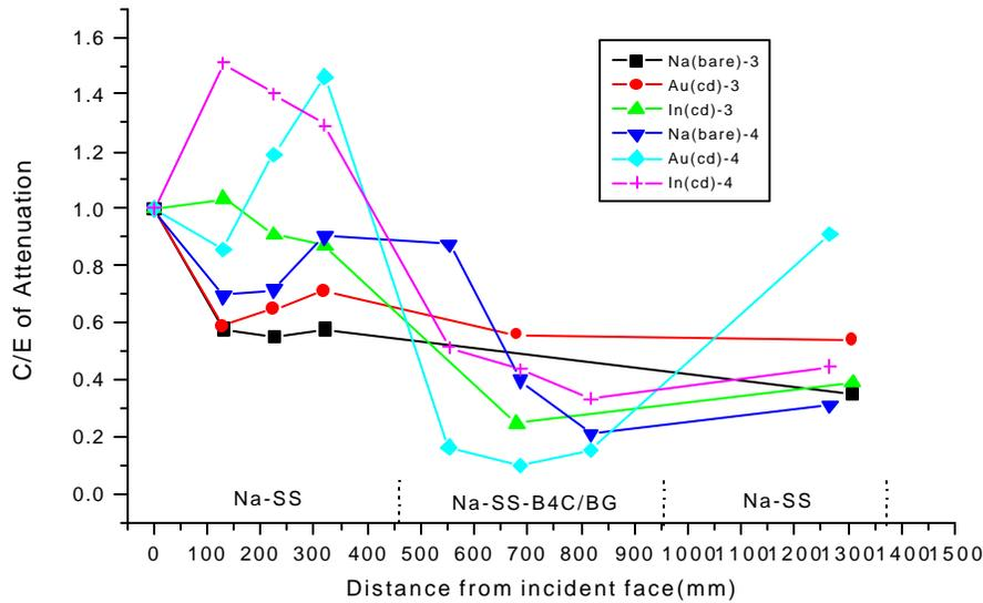
**Figure 7. C/E in transport through steel-borated graphite/boron carbide-sodium shields**
