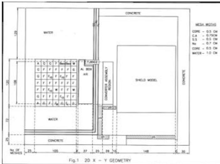
**Figure 5. Calculational 2-D Geometry** calculations, carried out elsewhere. Details of our calculations are given in Ref.15.
