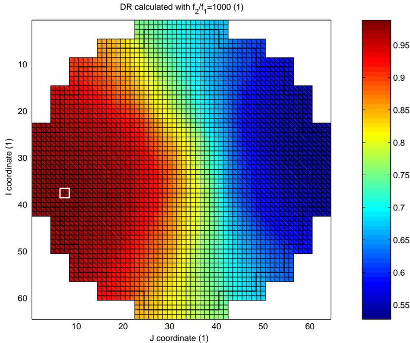
**Figure 3. Simulated radial space-dependence of the Decay Ratio in Forsmark-1 in case of a local noise source and a global noise source (the white square represents the location of the local noise source).**
