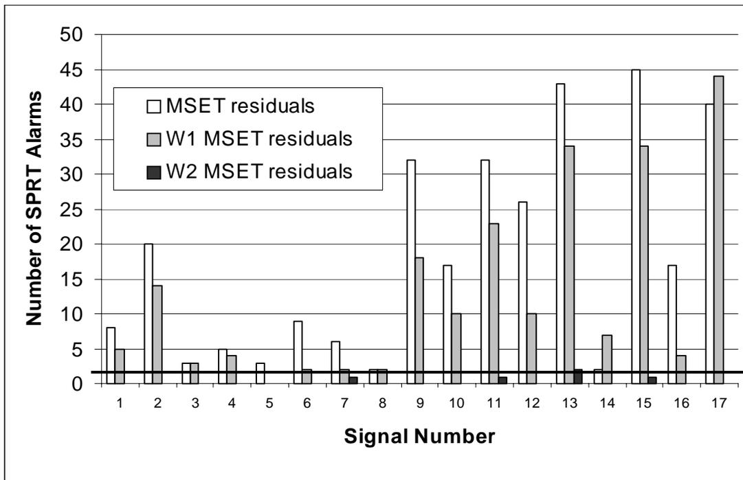
**Figure 2 – Comparison of SPRT alarms for the three Sets of MSET residuals. The bold horizontal line is the maximum expected number of false alarms for the data set based on a user-defined false alarm probability rate of  $10^{-3}$ .**
