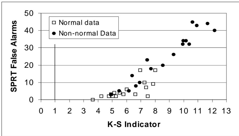
**Figure 3 – SPRT alarms vs. K-S indicator for normally and non-normally distributed residuals. A K-S indicator for serially-correlated data with a threshold of 3.5 is suggested for SPRT robustness.**
