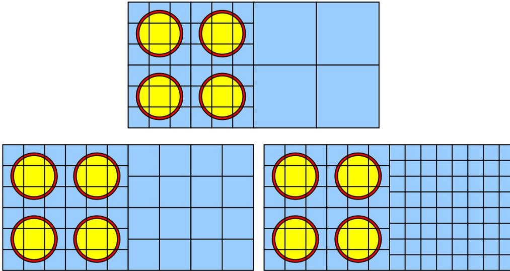
**Figure 3. Grid Schemes for Reflector Model Study in NEWT**
