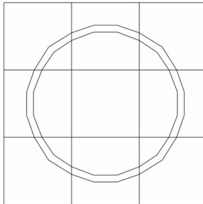
**Figure 2. NEWT Pin-Cell Discretization**
