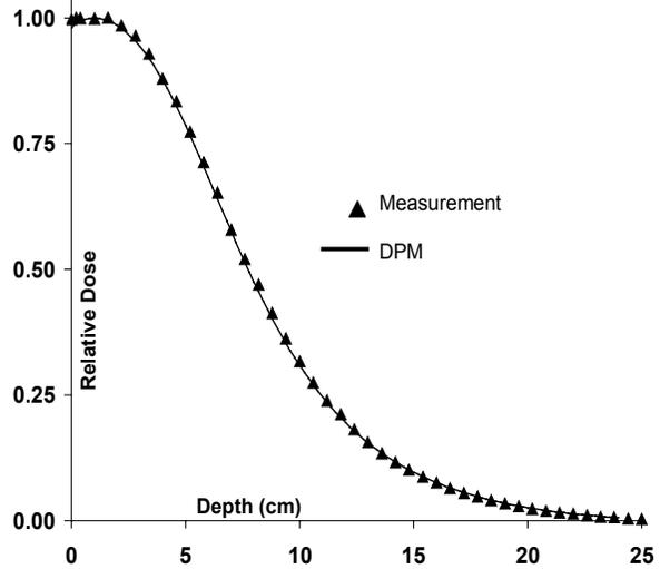
Figure 1 (b) Central axis depth dose comparison for 50 MeV electrons in water [9].
