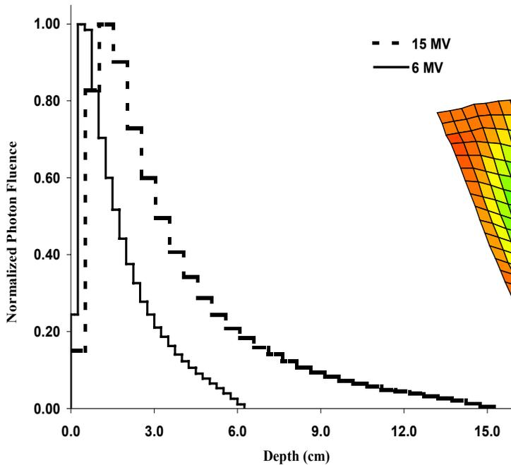
**Figure 3. Normalized photon fluence as a function of energy, along the central axis, for 6 MV, 15 MV photon beams.**
