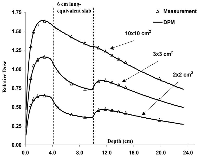
**Figure 6. Relative central axis depth dose for 15 MV photons incident on the inhomogeneous (solid-water/lung/solid-water) phantom.**
