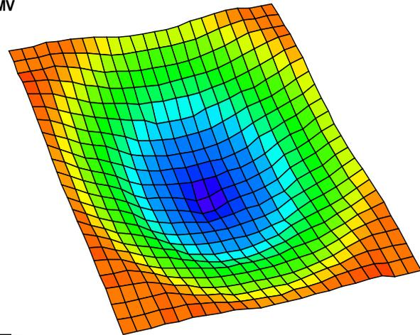
**Figure 4. The reconstructed, cartesian, virtual source fluence map for the 6 MV beam, illustrating the discrete photon fluence “elements”.**
