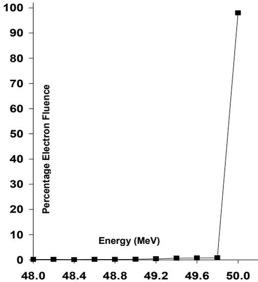
Figure 1 (a) Percentage electron fluence as a function of energy for the 50 MeV electron beam from the MCNP Monte Carlo treatment head simulation of the racetrack microtron [9].
