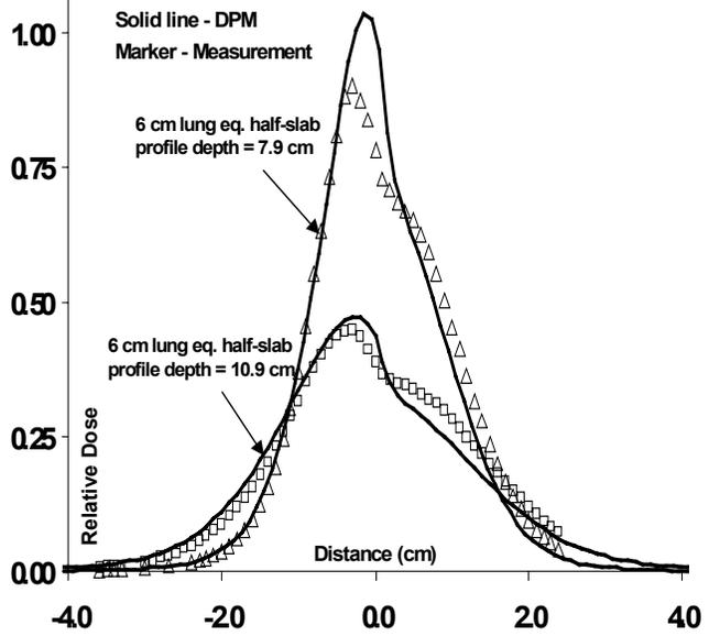
Figure 2 (b) Relative x-axis profile dose for 50 MeV electrons incident on a 6 cm lung-equivalent half-slab. Profiles are normalized to the area under the corresponding curve [9].
