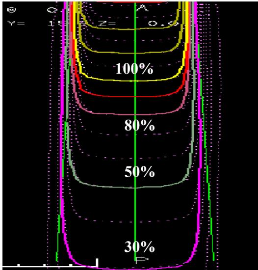
**Figure 4(a).** Relative transverse profile dose as a function of depth for the 6 MV,  $5 \times 5 \text{ cm}^2$  field.
