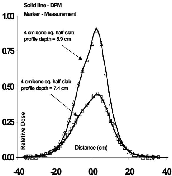
Figure 2 (a) Relative x-axis profile dose for 50 MeV electrons incident on a 4 cm bone-equivalent half-slab. Profiles are normalized to the area under the corresponding curve [9].
