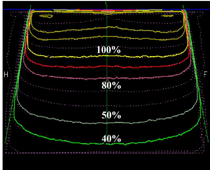
**Figure 4(b).** Relative transverse profile dose as a function of depth for the 6 MV,  $40 \times 40 \text{ cm}^2$  field.
