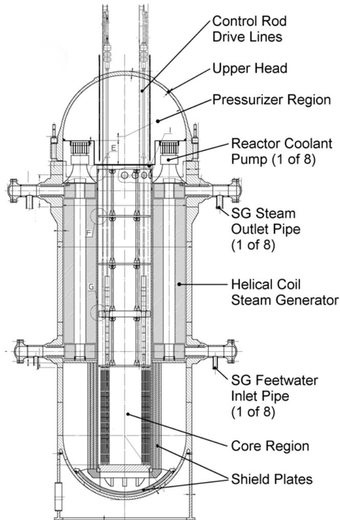
**Figure 1. IRIS integral vessel layout.**
