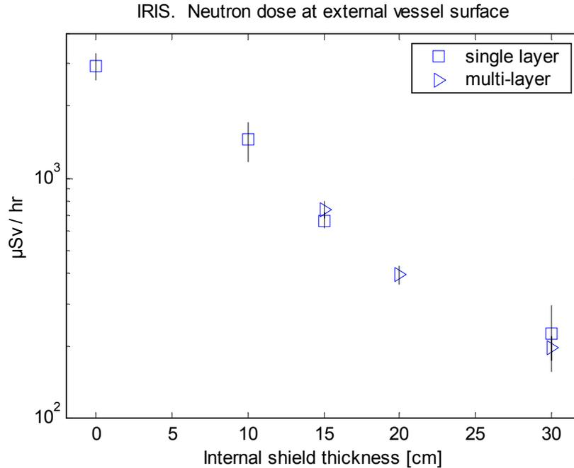
**Figure 5. Neutron dose outside vessel vs. steel shield thickness.**
