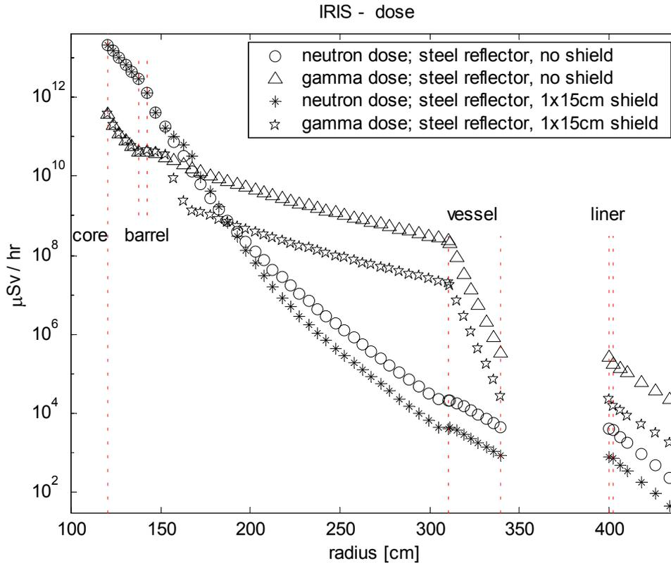
**Figure 4. Neutron and gamma doses for Cases 2 and 4.**
