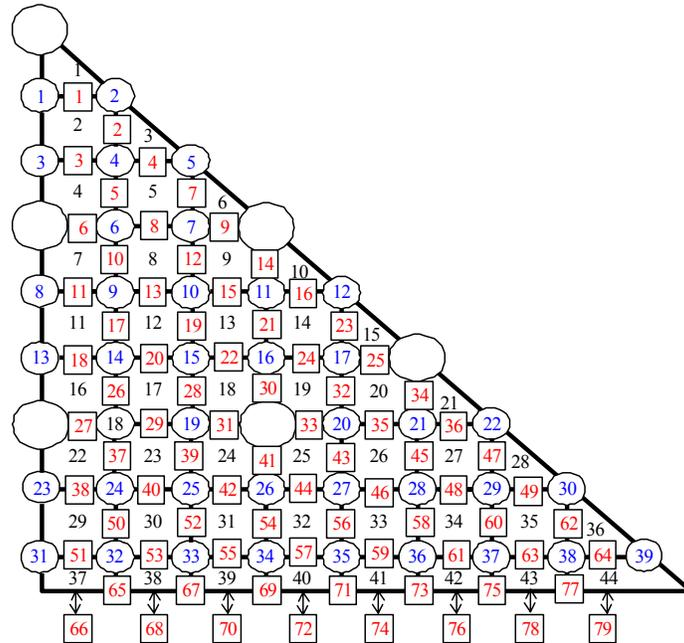
**Figure 4. Hot Assembly model for IRIS transient analyses (rods number in blue, channel numbers in black and gap numbers in red)**
