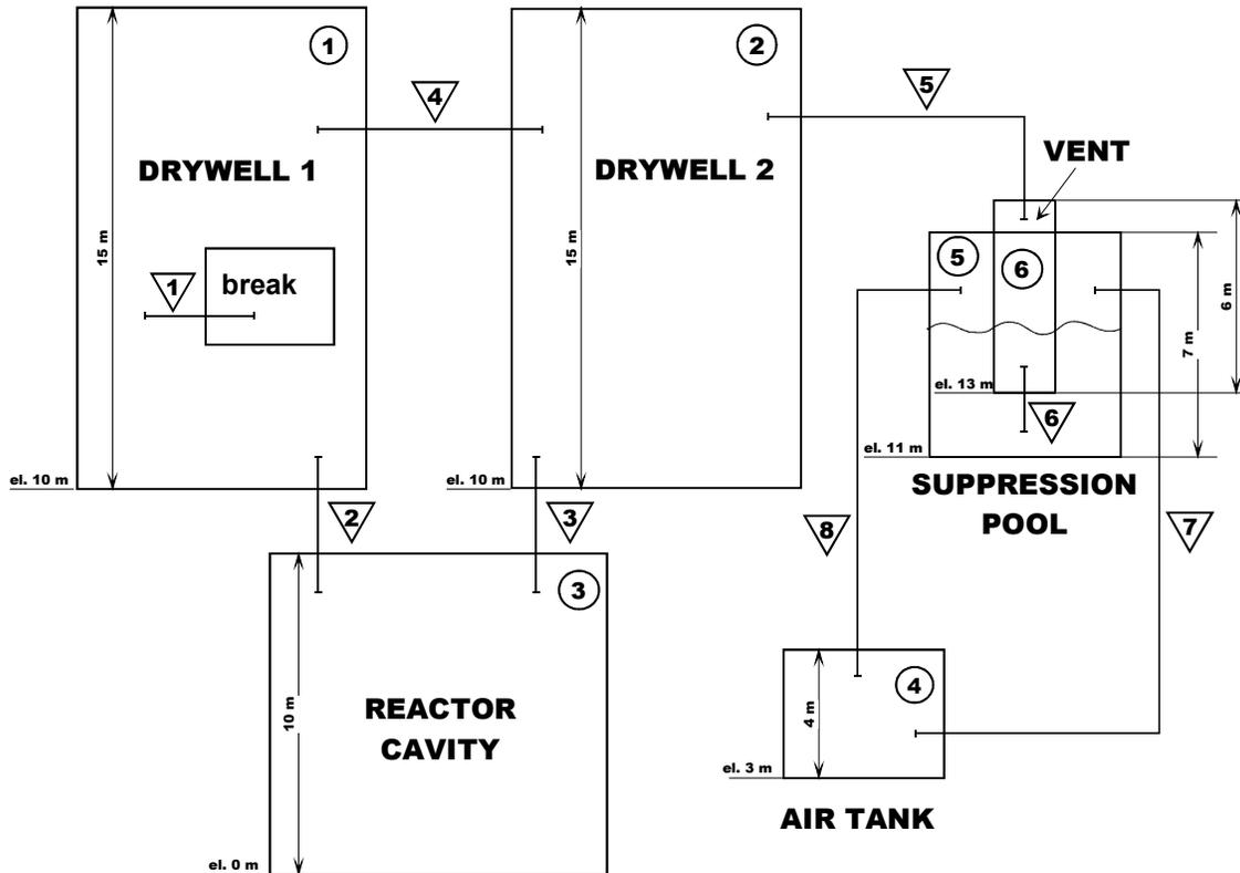
Figure 6. IRIS Simplified Containment Model for GOTHIC
