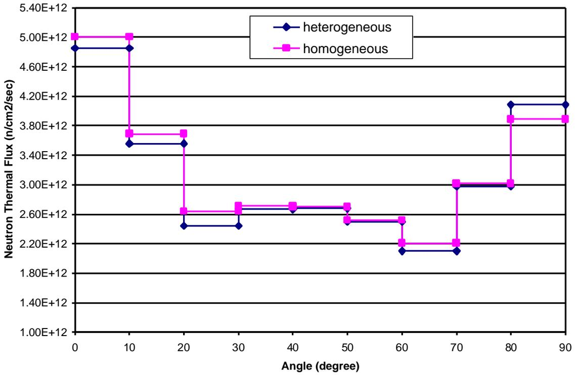
**Figure 5. Comparison of neutron thermal fluxes in the IRIS core barrel calculated using the heterogeneous and homogeneous XYZ core models.**
