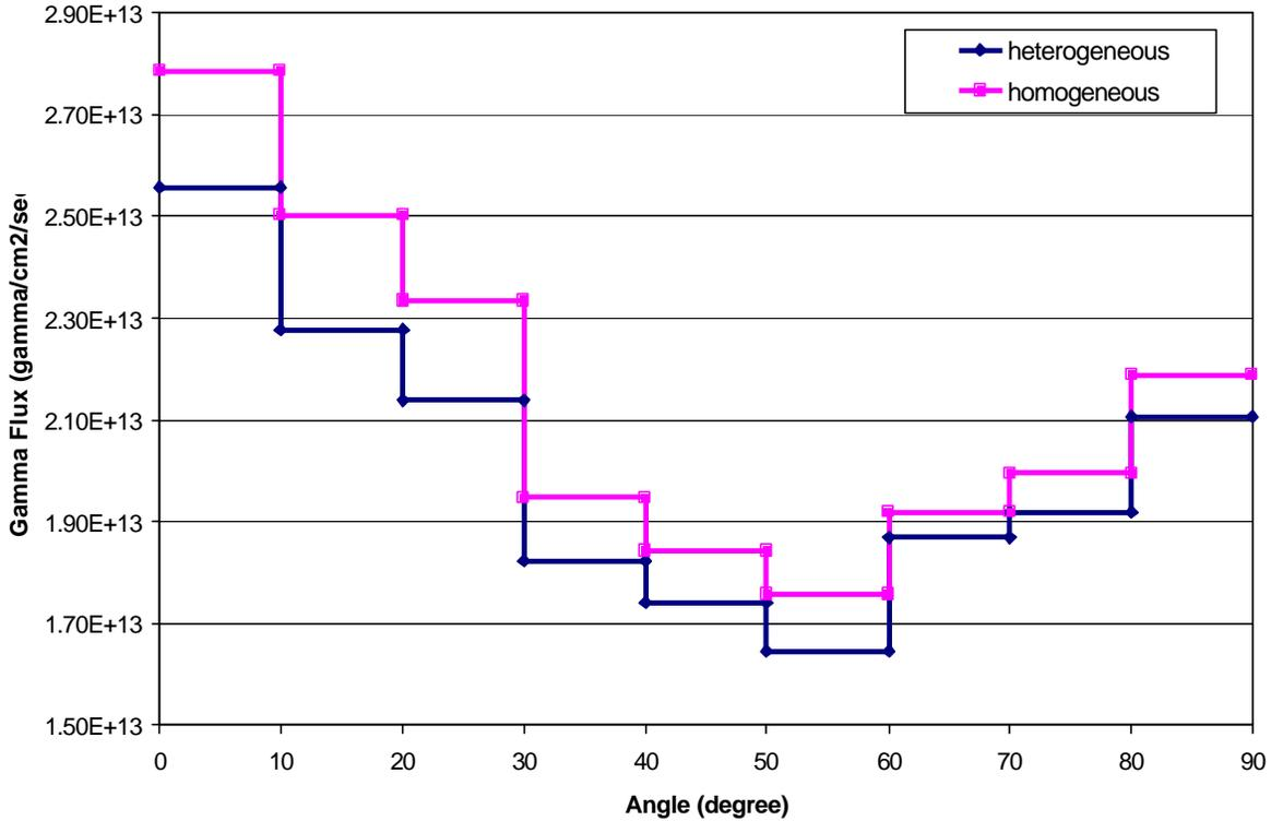
**Figure 9. Comparison of gamma fluxes in the IRIS core barrel calculated using the heterogeneous and homogeneous XYZ core models.**
