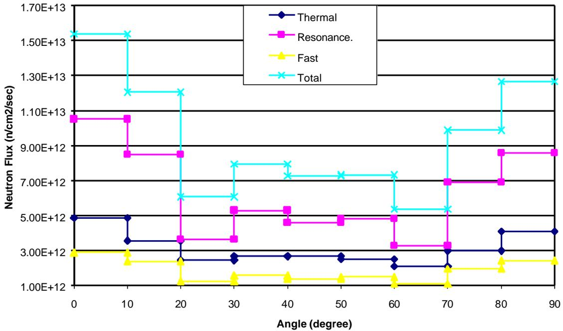
**Figure 3. Neutron flux in the IRIS core barrel for various azimuthal angles calculated using the heterogeneous XYZ core model.**
