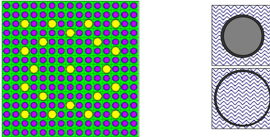
**Figure 2. Horizontal cross section of a 15x15 fuel assembly and of its unit-cells.**
