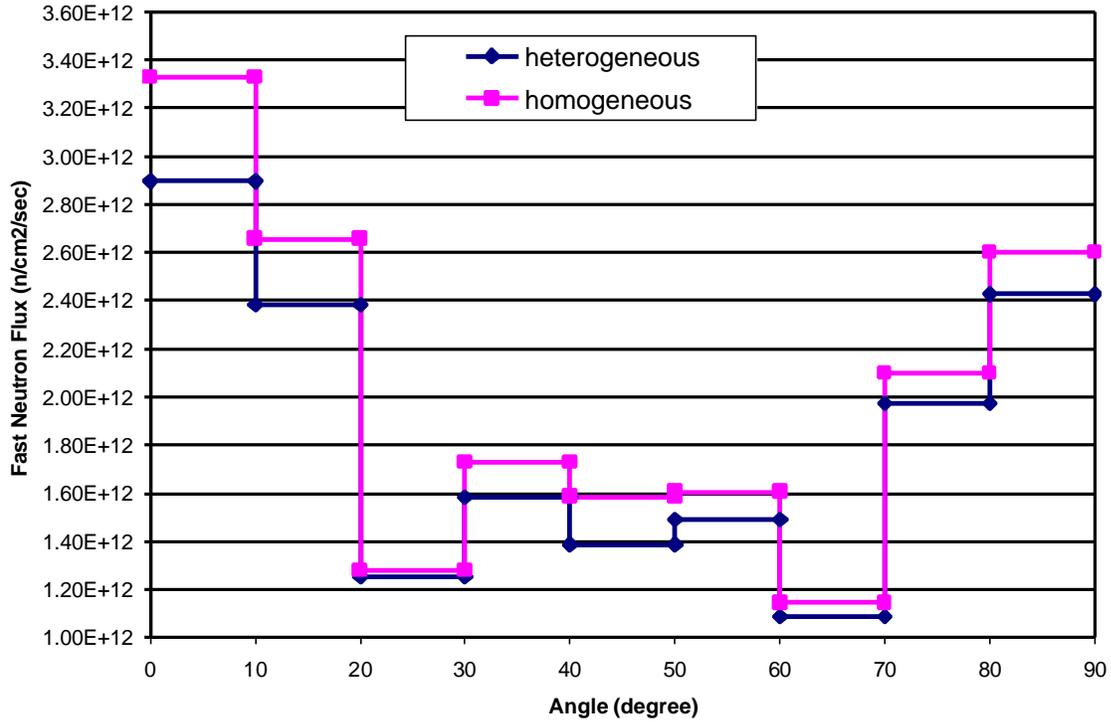
**Figure 7. Comparison of fast neutron fluxes in the IRIS core barrel calculated using the heterogeneous and homogeneous XYZ core models.**
