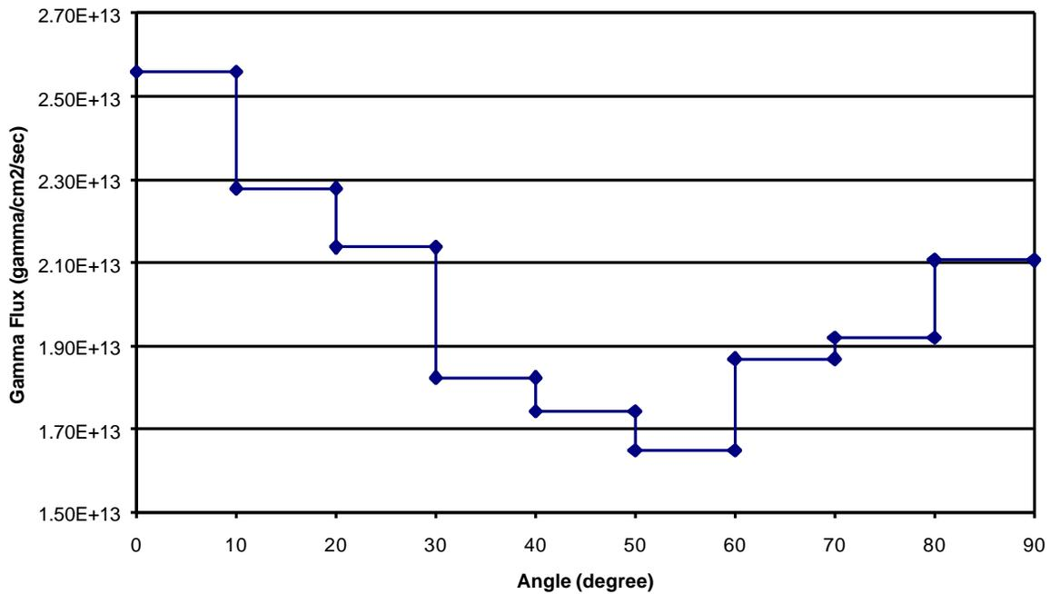
**Figure 4. Gamma flux in the IRIS core barrel for various azimuthal angles calculated using the heterogeneous XYZ core model.**
