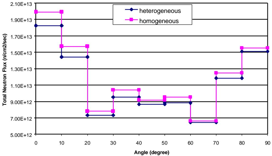
**Figure 8. Comparison of total neutron fluxes in the IRIS core barrel calculated using the heterogeneous and homogeneous XYZ core models.**
