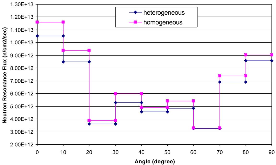
**Figure 6. Comparison of resonance neutron fluxes in the IRIS core barrel calculated using heterogeneous and homogeneous XYZ core models.**
