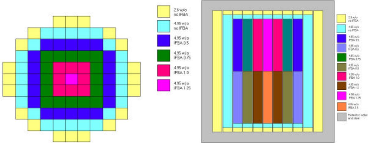
**Figure 1. IRIS Benchmark #44: Core configuration vertical and horizontal views including fuel enrichment and IFBA distribution.**
