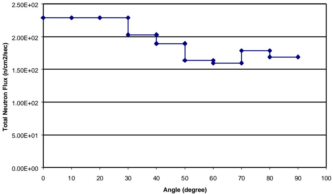
**Figure 11. Total neutron flux in IRIS RPV for various azimuthal angles calculated using the heterogeneous XYZ core model.**
