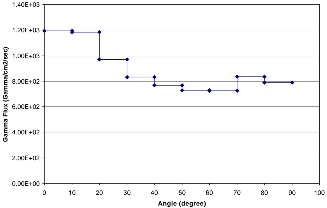
**Figure 10. Gamma flux in IRIS reactor PV for various azimuthal angles calculated using the heterogeneous XYZ core model.**
