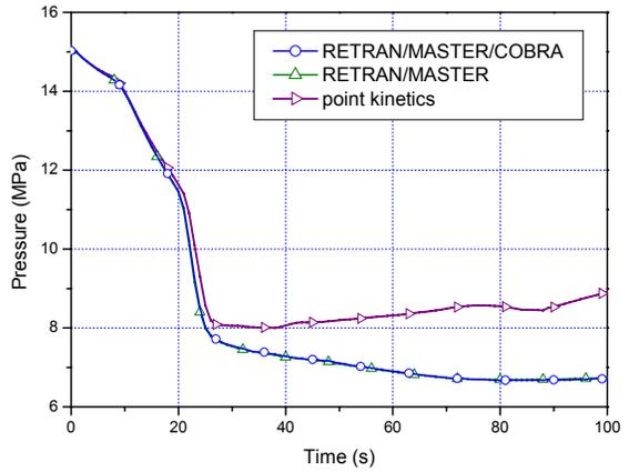
Figure 6. Pressurizer Pressures
