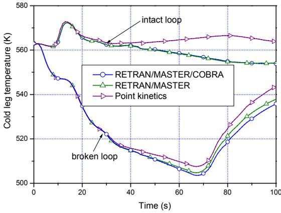
Figure 5. Coolant Temperatures for Cold Legs
