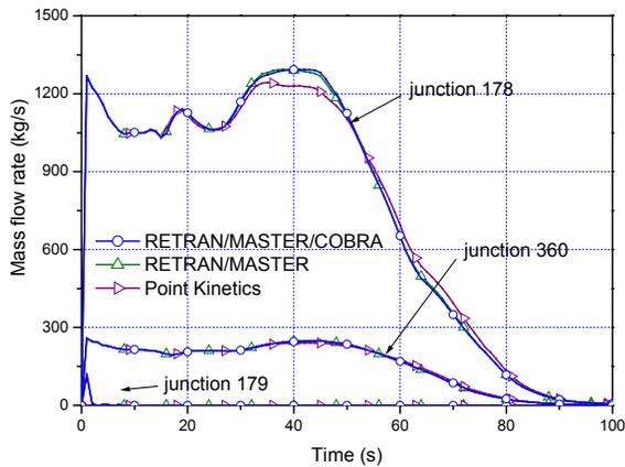
**Figure 3. Break Flow Rates**
