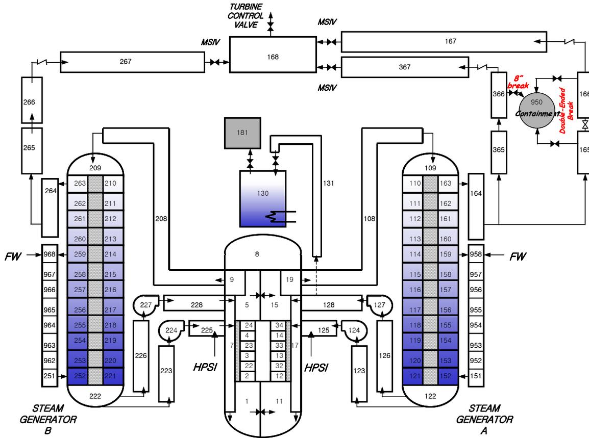
Figure 2. TMI-1 Plant NSSS System Nodalization for MSLB Benchmark Problem
