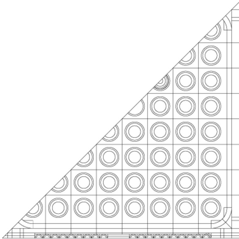
**Figure 1b: Computational mesh for linear cross sections.**
