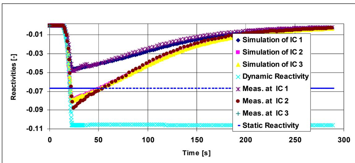
**Figure 5. IPK reactivities based on measured and calculated IC signals and static and dynamic reactivities at a given measurement in Paks NPP**
