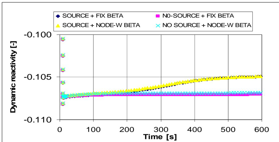
Figure 4. SCRAM with stuck CA. Effect of neutron source and node wise  $\beta$  on reactivity
