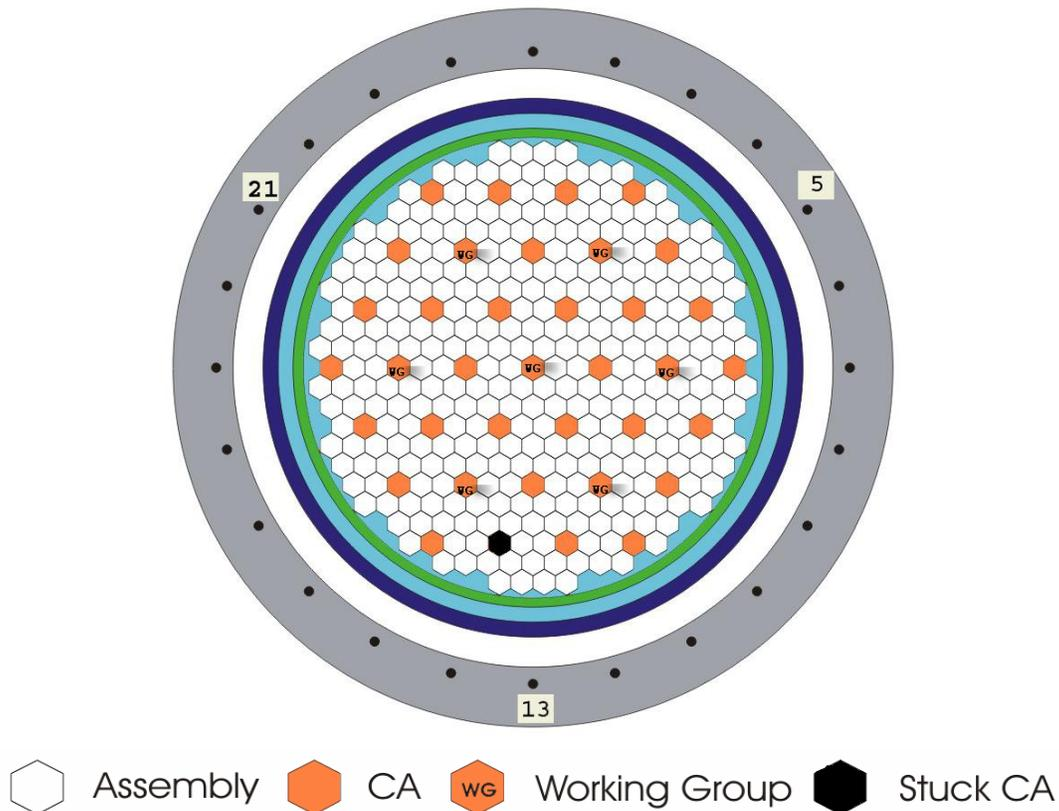
**Figure 1. Location of the Control Assemblies and the position of the ionization chambers used at the start-up measurements in a VVER-440 NPP**
