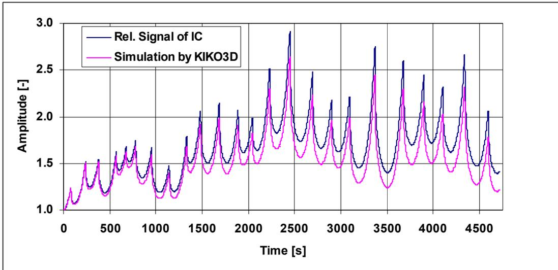
**Figure 10. Core amplitude and IC signal (upper curve) during simulated  $\partial\rho/\partial H$  measurement with KIKO3D Paks NPP Unit 3, Cycle 15**
