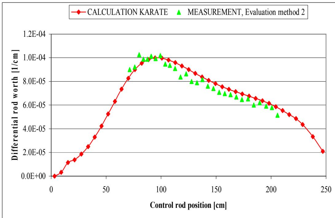
**Figure 13. Differential worth of Working Group derived from KARATE calculations and from the chosen evaluation methods of the measured IC signals.**
