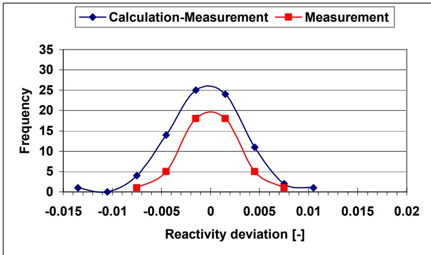
**Figure 9. Difference of Calculated and Measured Scram Rod Worths Paks NPP Unit 1-4**
