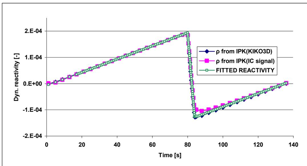
**Figure 12. IPK reactivity derived from core amplitude and IC signal together with fitted reactivity curves during simulated  $\partial\rho/\partial H$  measurement Paks NPP Unit 3, Cycle 15**
