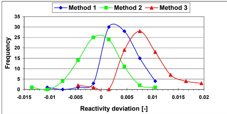
**Figure 8. Difference of Calculated and Measured Scram Rod Worths Paks NPP Unit 1-4**
