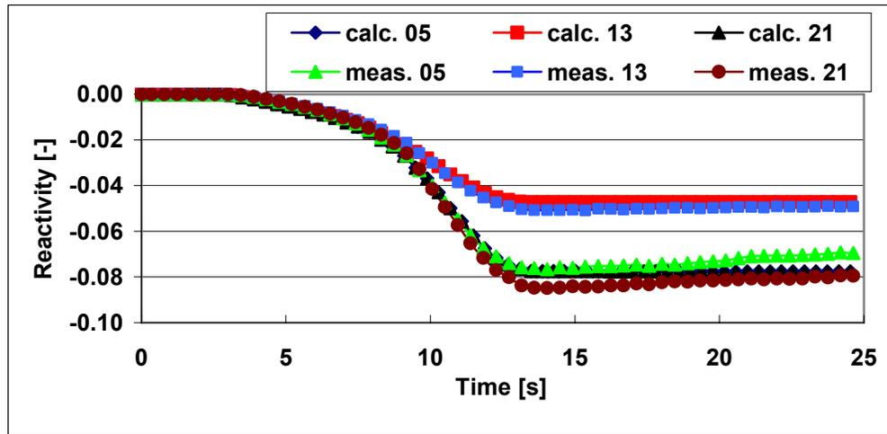
Figure 7. Calculated and Measured IPK Reactivities of IC signals, Paks NPP-1, Cycle 13
