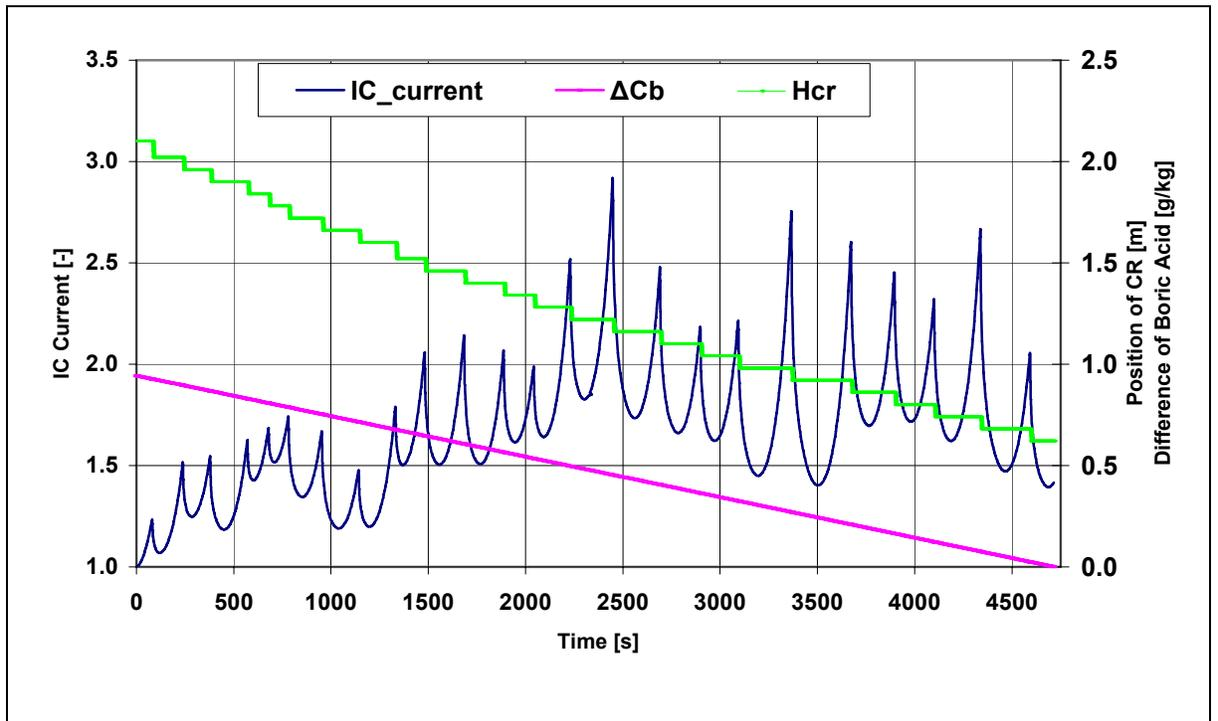
**Figure 3. Change of boric acid concentration, position of working group and the current of the ionization chamber during the  $\partial\rho/\partial H$  measurement being simulated**
