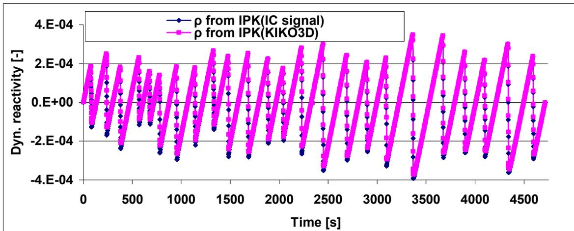
**Figure 11. Inverse point kinetic reactivity derived from core amplitude and IC signal during simulated  $\partial\rho/\partial H$  measurement with KIKO3D Paks NPP Unit 3, Cycle 15**
