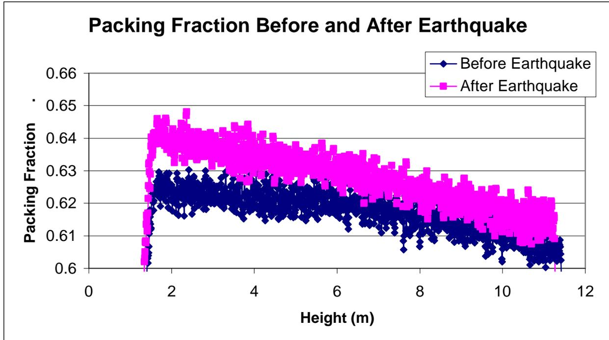
**Figure 2 Before and After Earthquake Packing Fraction**
