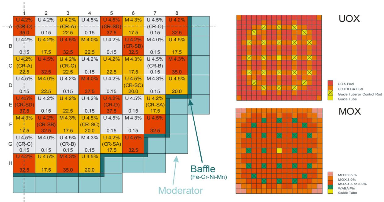
**Figure 3. Core configuration and fuel assembly layout for the  $\text{UO}_2$  and MOX assemblies of the PWR MOX/ $\text{UO}_2$  core transient benchmark. In the core configuration, CR-A to CR-D denote four different control rod banks, and CR-SA to CR-SD refer to four shutdown rod banks. Reflective boundary conditions apply along the dashed symmetry lines.**
