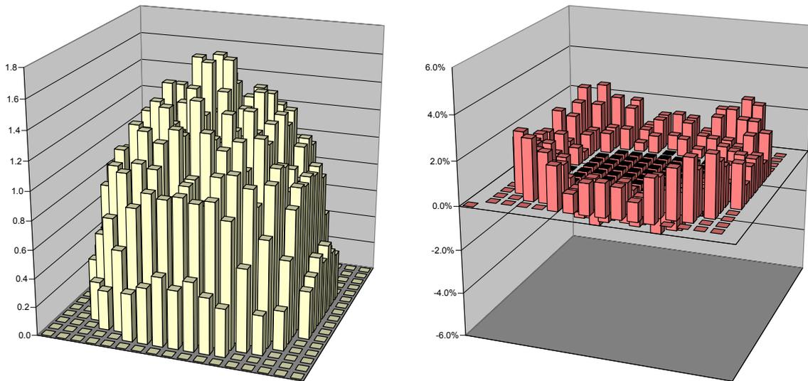
**Figure 4. Left: Normalized whole core assembly power distribution of the ARO reactor state obtained from the MCNP solution with JEF-2.2 point data. Right: Relative deviations between the distribution from the DORT S<sub>4</sub>-P<sub>1</sub> calculation using pin cell homogenized 16-group cross sections and the MCNP solution.**
