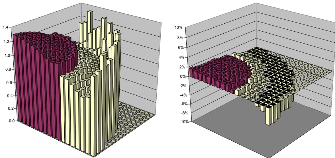
**Figure 2. Radial fission rate distribution for one quarter of the VENUS-7/0 configuration. Left: Pin fission rates calculated with MCNP. Right: Relative differences between the MCNP and THREEDANT results. The values for the inner MOX and the outer  $\text{UO}_2$  zones are displayed in different colors.**
