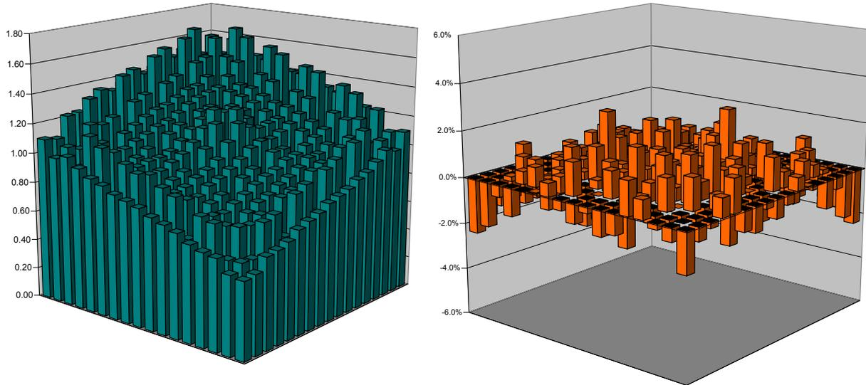
**Figure 5. Left: Normalized pin-wise power distribution of assembly F6 of the ARO reactor state obtained from the MCNP solution with JEF-2.2 point data. Right: Relative deviations between the distribution from the DORT  $S_4$ - $P_1$  calculation using pin cell homogenized 16-group cross sections and the MCNP solution.**
