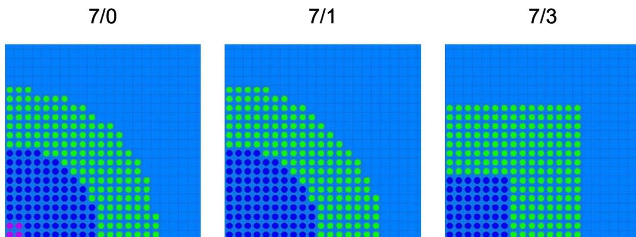
**Figure 1. Horizontal cut through one quarter of the VENUS-7 assemblies. Blue pins: MOX fuel; green pins:  $UO_2$  fuel. In assembly 7/0, the central pins for the substitution experiments are displayed in magenta.**
