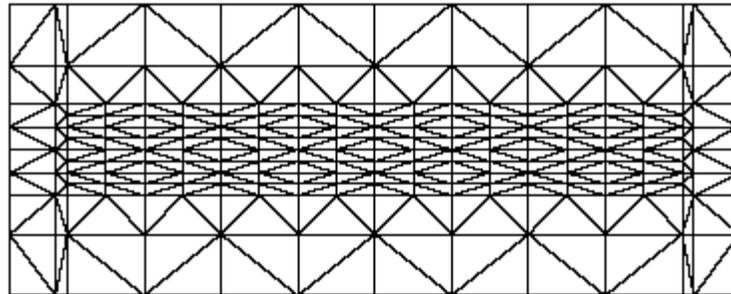
**Figure 3 : 2D mesh organisation for domains 5 to10 from fig.6. The number of refined elements must be a multiple of 4 and a special size layer must be placed between refined and initial size elements.**
