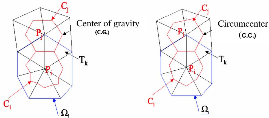
**Figure 1 : Dual meshes for FVFE method : gravity center (left), circumcenter (right)**
