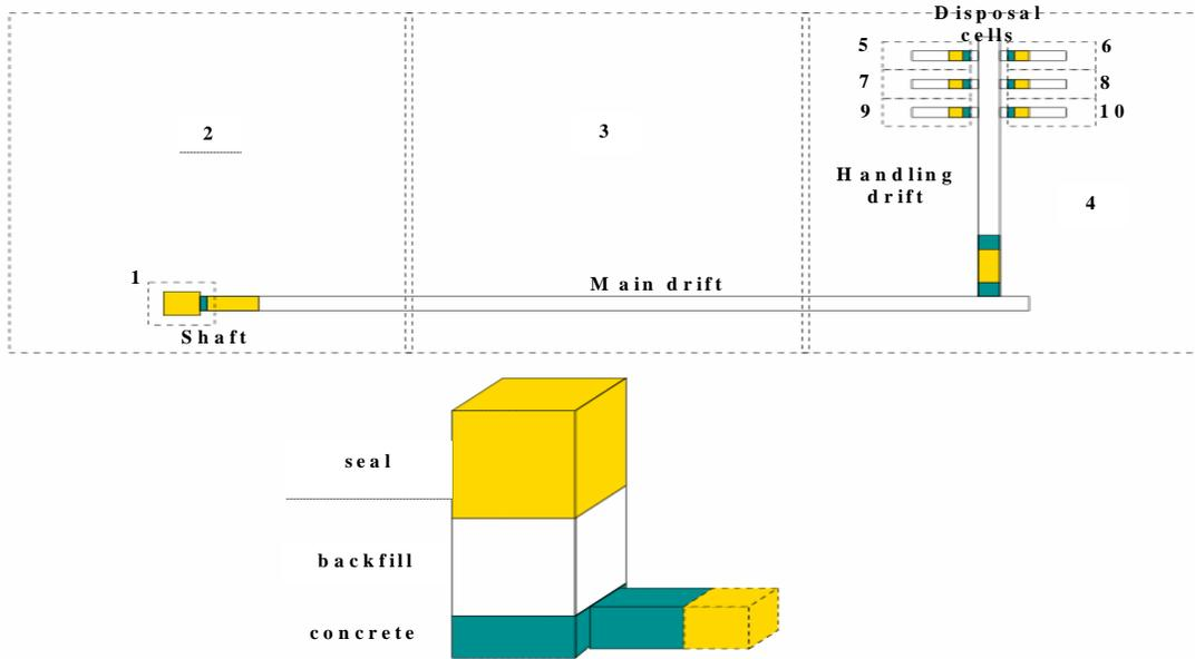
**Figure 6 : Repository system and the shaft - 10 embedded meshes**
