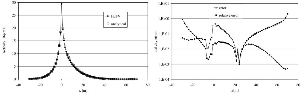
**Figure 5** A sample test case for the FVFE method. Activity profile passing through the continuous point source (left) and the corresponding errors (right).
