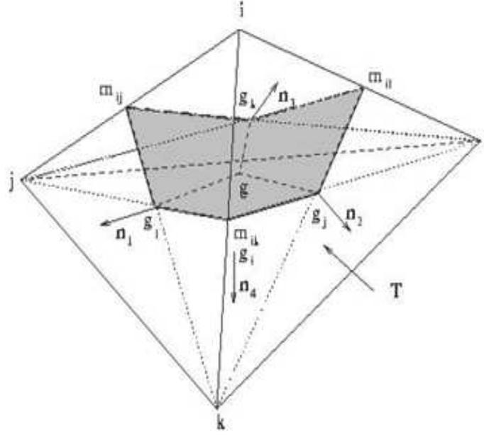
**Figure 2 : Dual mesh included in T, constructed by the CG method**
