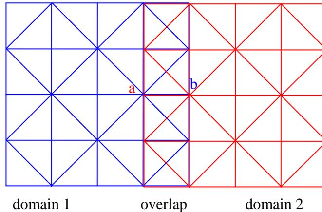
**Figure 4 : Principle of domain decomposition with the overlap thickness of one layer.**
