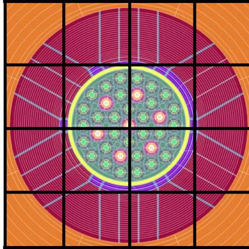
**Figure 2. Decomposition in 16 subdomains for the JHR core.**
