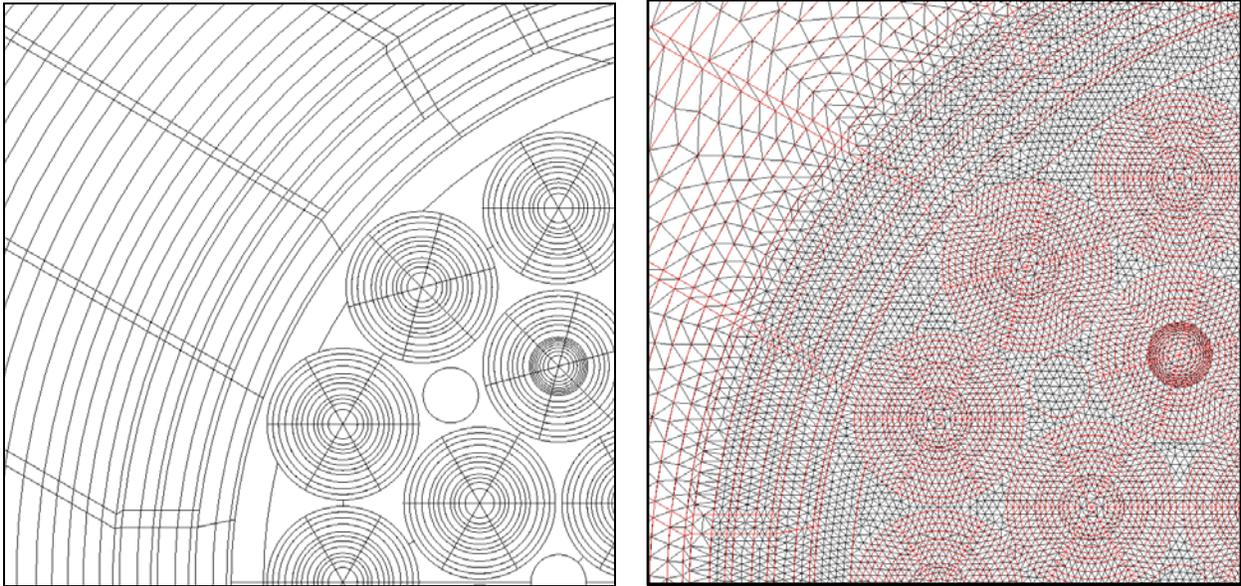
**Figure 1. Part of the physical domain and its discretization by a triangular mesh**
