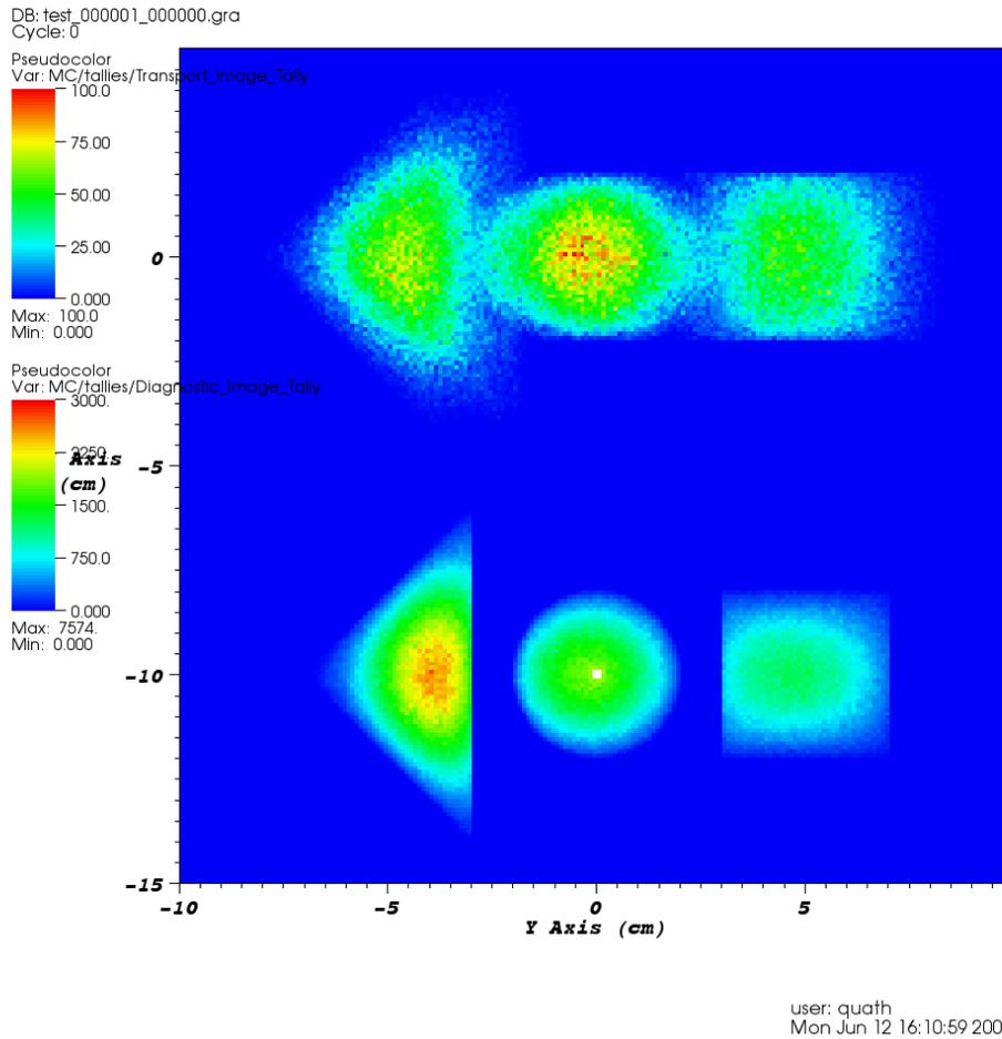
Figure 2. Comparison of a regular transport (top) and biased transport (bottom) tally.
