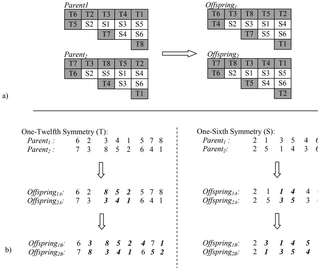
**Figure 5. Example of recombination operator using PMX method on one-sixth and one-twelfth symmetries fuel assemblies: a) Real core loading pattern. b) Equivalent chromosomes with genes string.**
