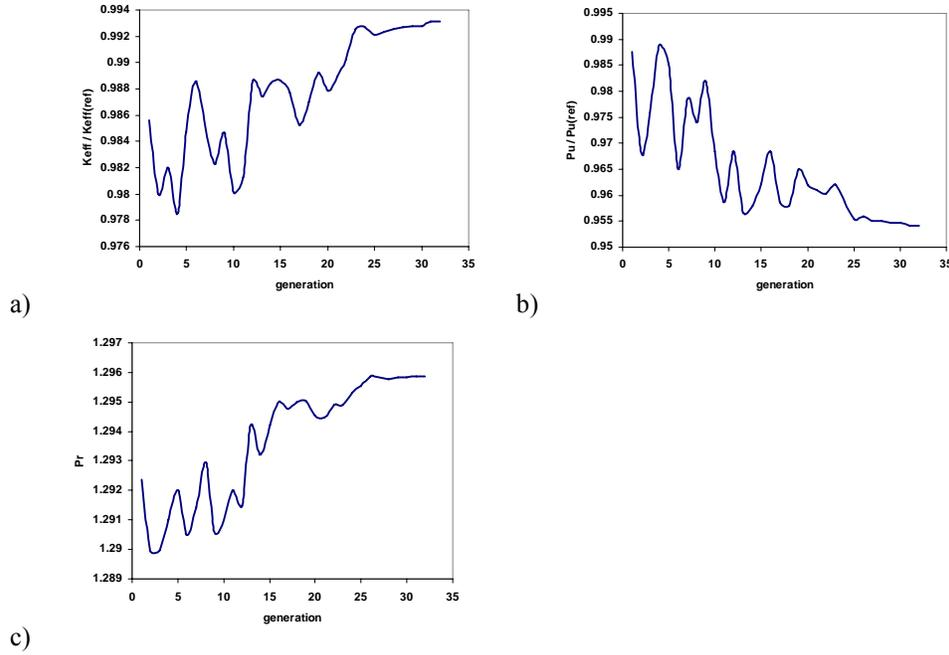
**Figure 7. Evolutions of the effective multiplication factor ( $K_{eff}$ ), power peaking factor ( $P_r$ ) and remained plutonium concentration at EOC ( $Pu$ ) of the core versus generations: a) Relative  $K_{eff}$  of the core compare to reference equilibrium cycle loading pattern. b) Relative  $Pu$  compare to reference equilibrium cycle loading pattern. c) Exact  $P_r$  of the core**
