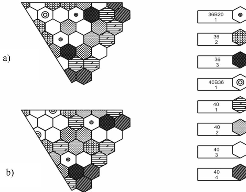
**Figure 8. Comparing the one-sixth core loading pattern design calculated by our approach to minimize the remained plutonium at EOC conditions with the reference cycle pattern: a) reference core loading pattern. b) proposed core loading pattern. The right column shows different fuel assemblies and year of burnup.**
