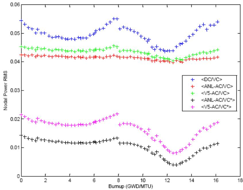
**Figure 4. Nodal power RMS as a function of burnup.**
