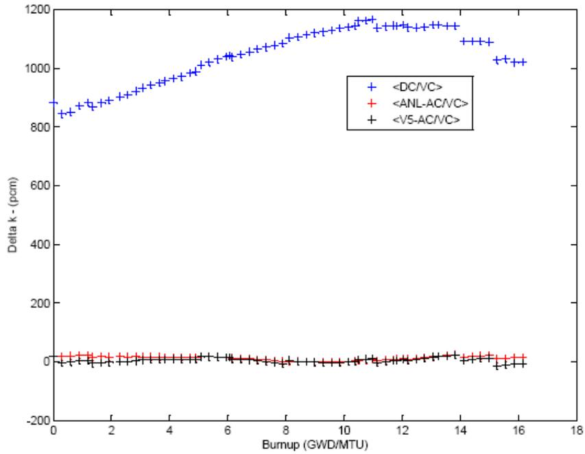
**Figure 3. Reactivity difference as a function of burnup.**
