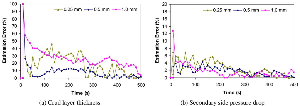
**Figure 4. Estimation errors for 25% decrease in thermal conductivity of Inconel.**
