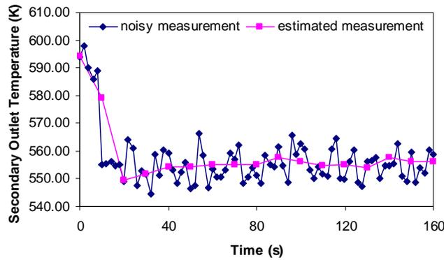
**Figure 2. Simulated and estimated measurement for 0.5 mm crud thickness and 50% decrease in thermal conductivity of Inconel.**
