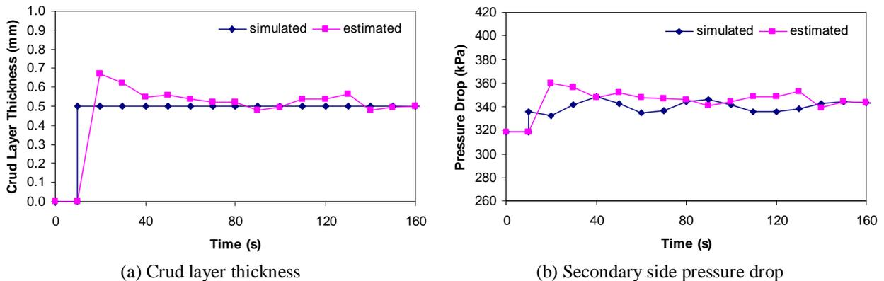
**Figure 3. Simulated and estimated component and system states for 0.5 mm crud thickness and 50% decrease in thermal conductivity of Inconel.**
