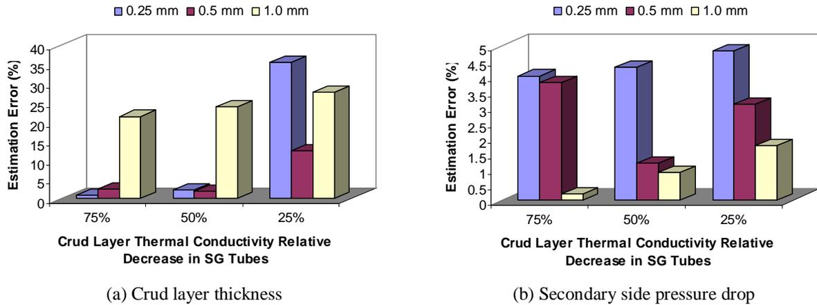
**Figure 5. Estimation errors for various crud thicknesses and thermal conductivities at 160 seconds.**
