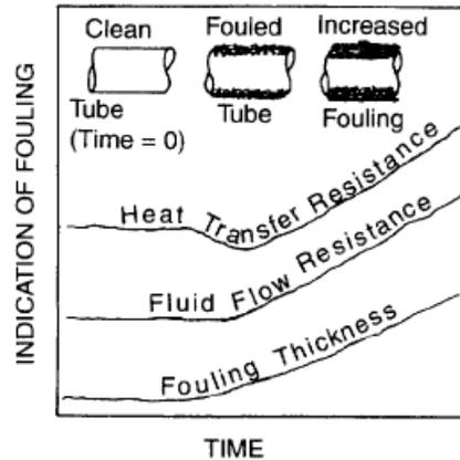
**Figure 1. The progression of fouling with time [3].**
