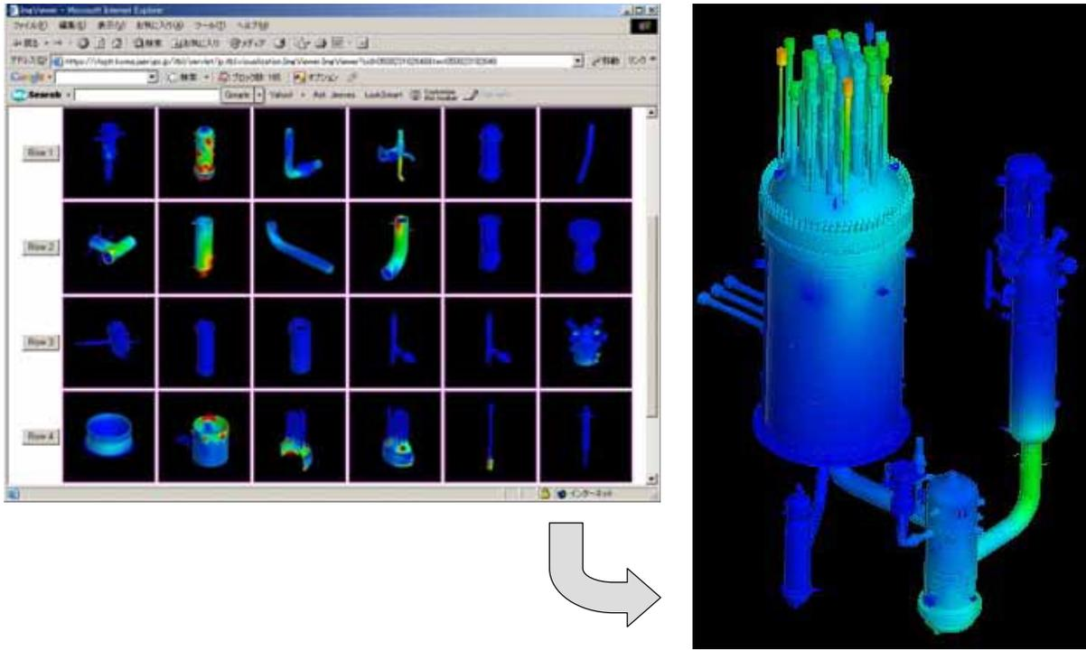
Figure 11. Static Analysis for Assembly Structure
