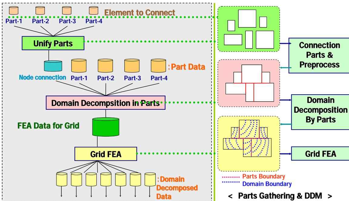
Figure7. Procedure of Assembly Analysis in FIESTA
