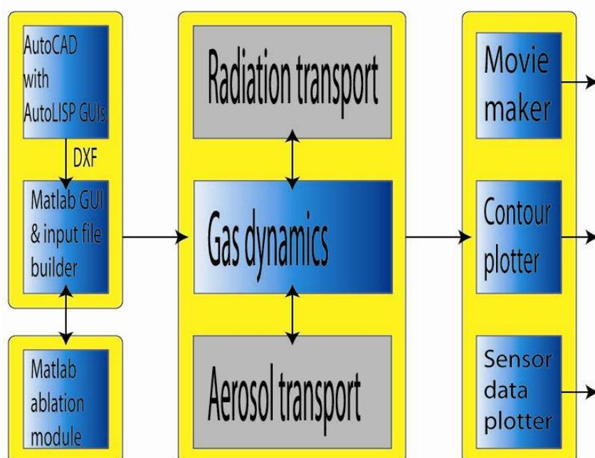
**Figure 1. Architecture of Visual Tsunami 2.0: pre-processor tools (left), MATLAB core (center), and MATLAB post-processor [2]. The implementation of radiation and aerosol transport models is left for future work.**
