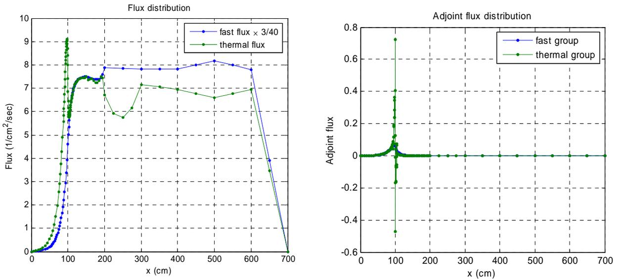
Fig. 6. Flux distribution, goal-oriented calculation, current as quantity of interest at  $x = 100$ , tolerance = 1% (Test Problem #3). Left = direct flux, right= adjoint flux.
