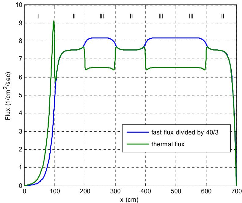
Fig. 1. Fast and Thermal Flux distributions (tolerance =  $10^{-5}\%$ ), Test Problem #1.
