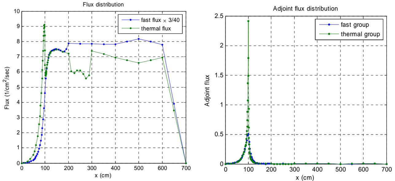
Fig. 5. Flux distribution, goal-oriented calculation, flux as quantity of interest at  $x = 100$ , tolerance = 1% (Test Problem #2). Left = direct flux, right= adjoint flux
