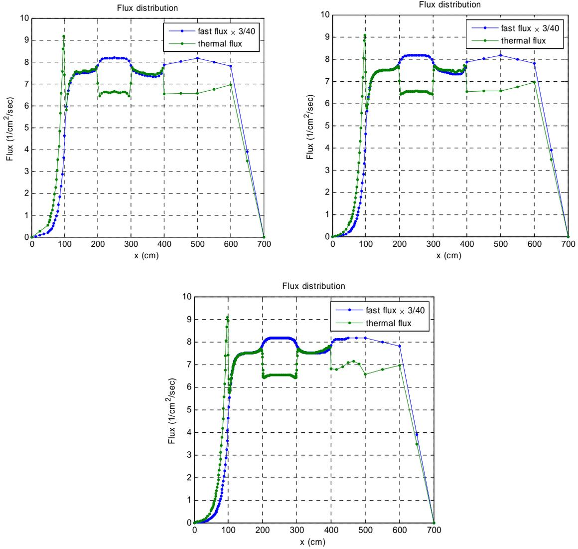
Fig. 2. Flux distributions, goal-oriented calculation, flux as quantity of interest in  $100 \leq x \leq 300$  (Model Problem B1). Tolerances used: top-left = 1%; top-right = 0.1%; bottom = 0.001%.
